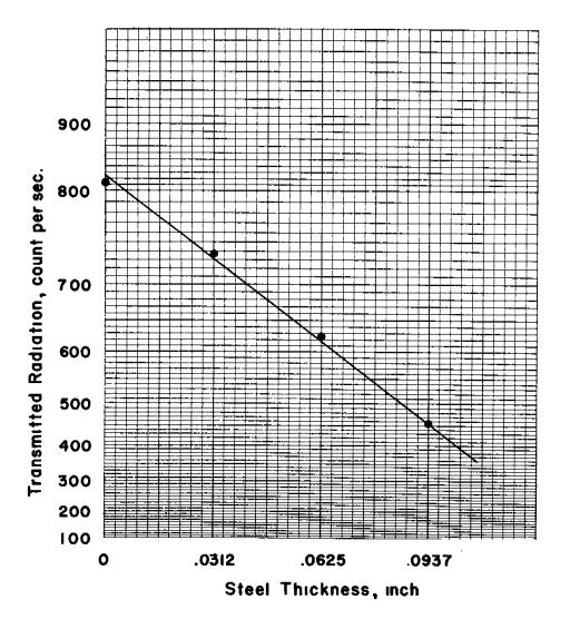
NP/45 L017386 NOTS CHINA LAKE, CALIFORNIA FIGURE 16. TRANSMITTED RADIATION VS. STEEL THICKNESS. ("VOID" DEPTH) 12 APRIL 1956 UNCLASSIFIED
