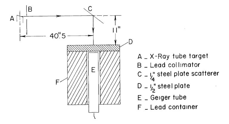
Diagrammatic Arrangement of Geiger Counter and X-ray Source
