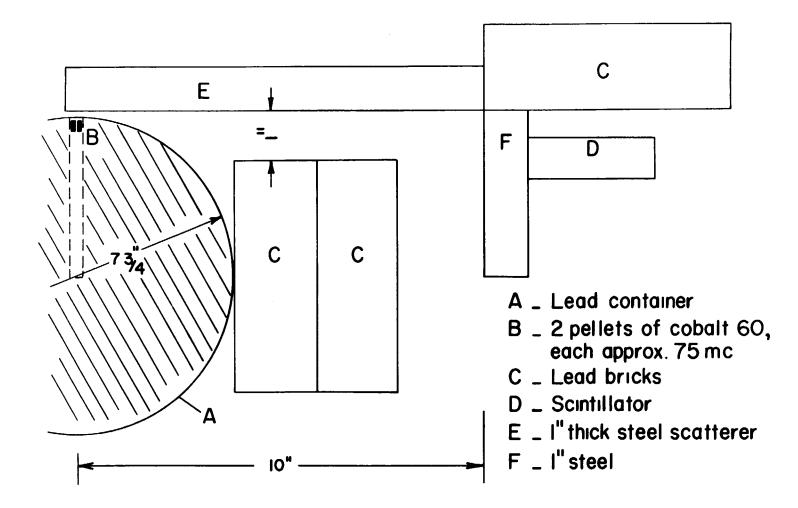
Diagrammatic Arrangement of Scintillator in connection with Gamma Radiation
