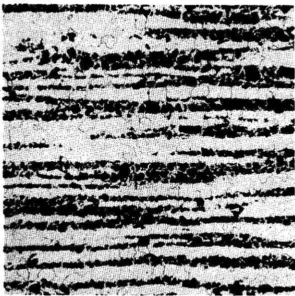
(a) Annealed structure of Heat 1764, soaked at 2300°F. 1/4 hour before forging and rolling.
