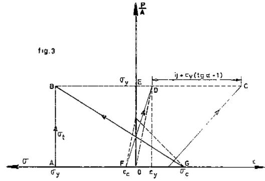
FIG. 12c. On the left side diagram  $\sigma$  versus nominal stress, for notched specimen with residual stresses of yield point value.
