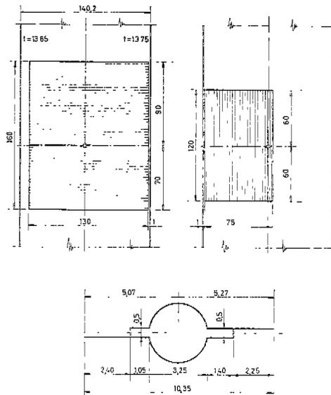
FIG. 3. SPECIMEN WITH SHORT CRACK.
