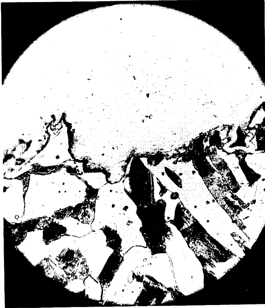
Fig. 11 - The Fracture at the back of the Specimen Steel E. (Cf. Fig. 7 & 8). Nital Etch x 600.
