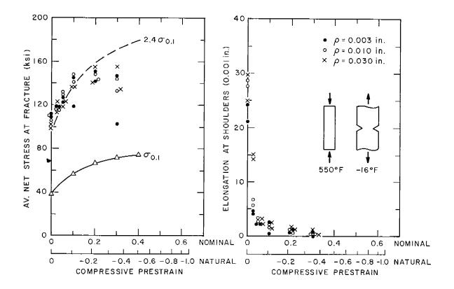
Fig. 15 Bars Axially Precompressed At 550°F, Side - Notched And Tested At -16°F.
