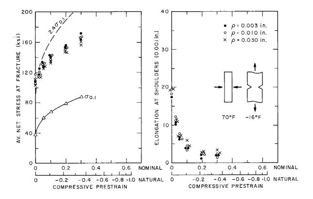
Fig. 14 Bars Laterally Precompressed At 70°F, Side - Notched And Tested At -16°F.
