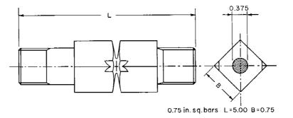
Fig. 6a Grooved Specimen.
