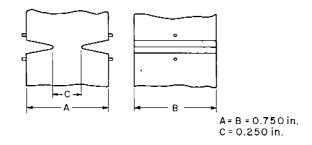
Fig. 6c Symmetrically Side-Notched Specimen.
