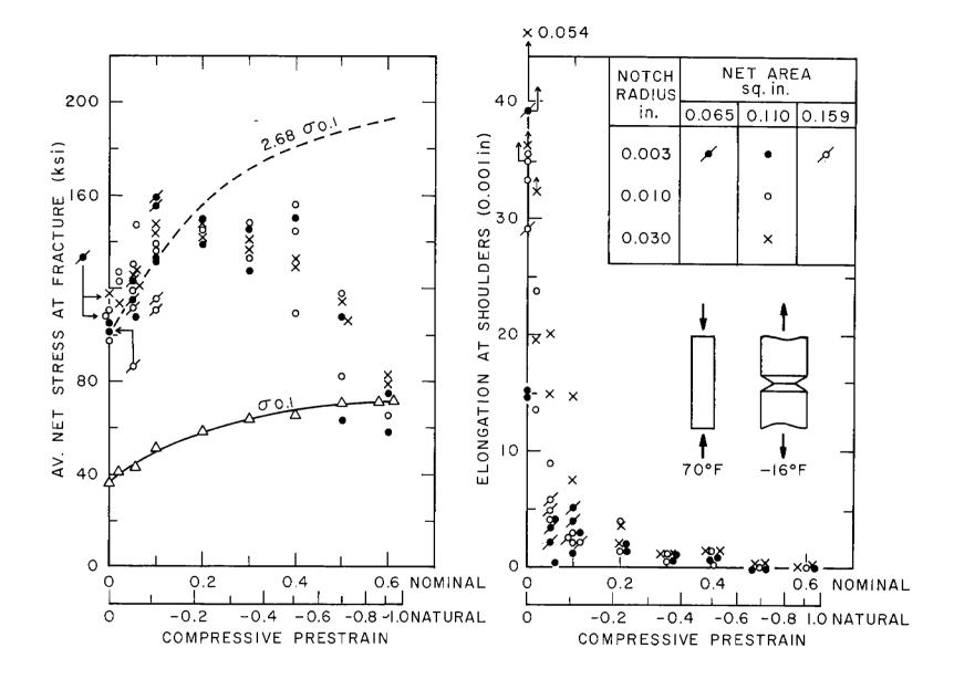
Fig. 8 Bars Axially Precompressed At 70°F, Grooved And Tested At -16°F.
