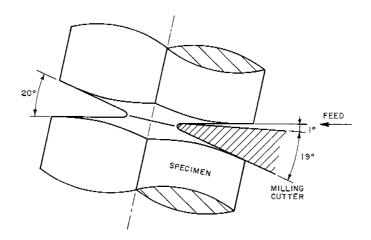
Fig. 6b Detail Of Groove Machining.
