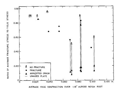
Fig. 3 Tests At -16°F Of 10 in. ABS-B Plates Compressed After Notching Initial Yield Stress 34 ksi.
