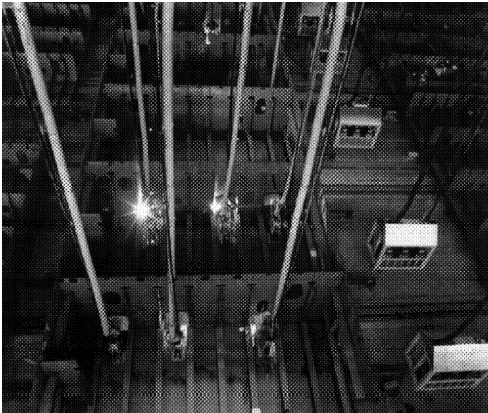
Figure 10 Structural Block For Double Hulled VLCC Being Welded Using Hirobo Robots At Odense, Lindo
