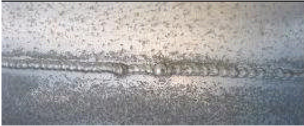
Fig. 1: Corrosion at a weld in 5xxx-series plate.
