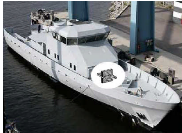
Fig. 1: Naval vessel in sandwich construction, illustrating typical location of X-joint
