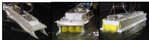
Fig. 3: Left: Catamaran Mode; Center: SWATH Mode; Right: Shallow Draft SES Mode
