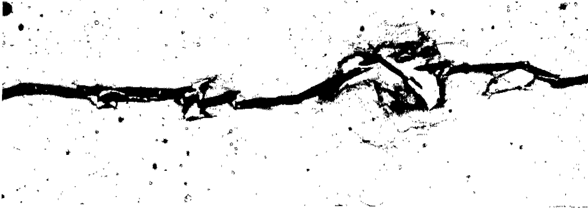
Fig.7. PLASTIC DEFORMATION ASSOCIATED WITH CLEAVAGE FRACTURE ON THE PLATE MIDSECTION OF Fe-3Si SPECIMEN 3Q-16. 150X
