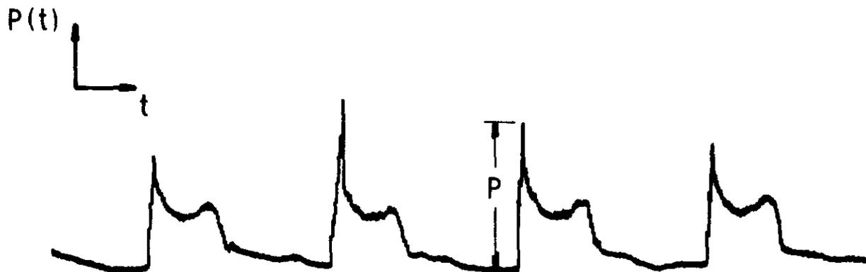
(a) Impact pressure traces for resonant sloshing with large amplitude hydraulic jumps or traveling waves
