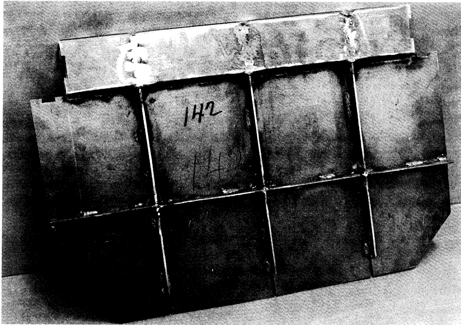
Fig. 16 - Transverse Bulkhead with Stiffening and Transverse Box
