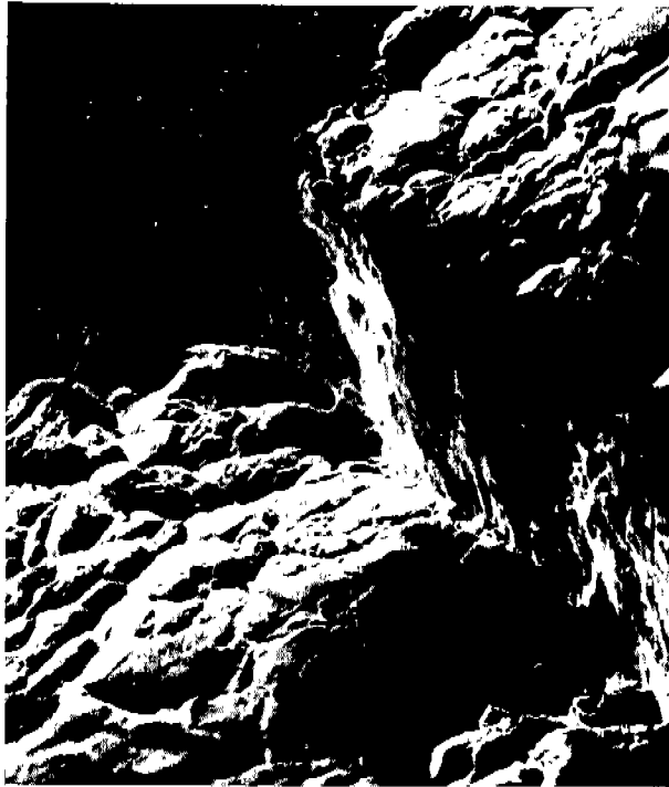
Fig A-5 Electron scanning micrograph giving 3-dimensional view of shear wall X200.
