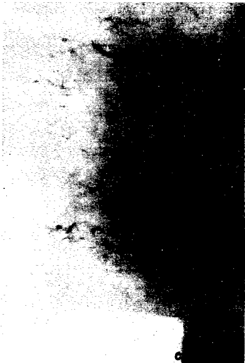
FIG. 3 - Illustration of Shrinkage, Type 1, Category C, Severity level 5 - from ASTM E-186, Reference Radiographs for Steel Castings.
