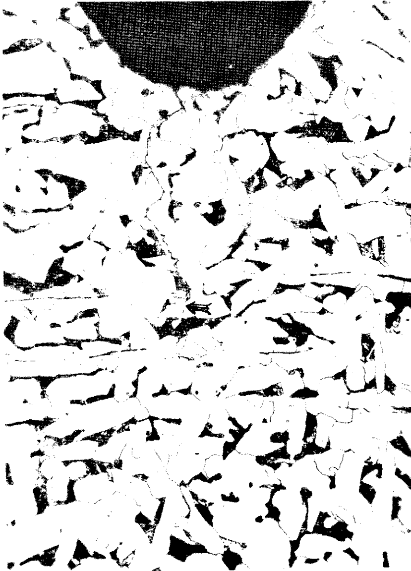
FIG: 17 - PHOTOGRAPH OF FATIGUE CRACK IN STEEL B; 27,500 psi, 100,000 CYCLES. 270X
