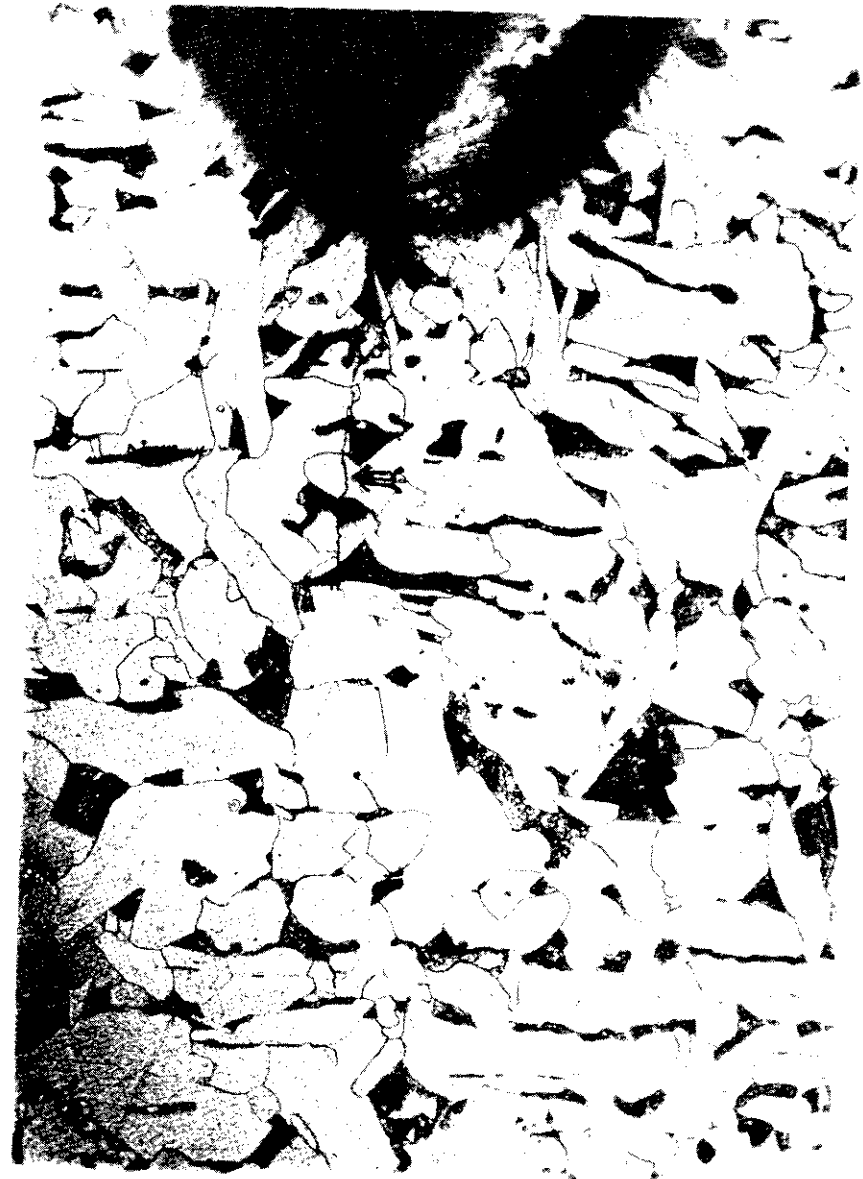
FIG. 20 - PHOTOGRAPH OF FATIGUE CRACK IN STEEL B 23,200 psi, 80,000 CYCLES. 270X
