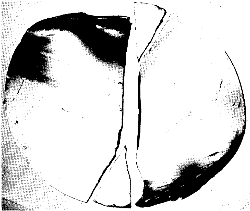
Fig. 13. Plan View of Fractured Disk #W-28 with Center Nib
