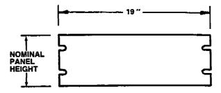
Consoliners may be used as storage, transit or permanent housing for 19" rack equipment with panel heights from 5%" to 26%" high. Like most TA cases, Consoliners are watertight and can be produced to conform to any applicable military specification.
