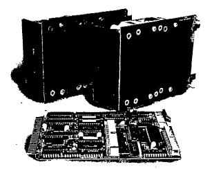
The ZT 8850 Winchester/Floppy Disk Controller with the ZT 8851 Floppy Disk Drive and ZT 8852 Winchester Disk Drive.
