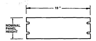
Consoliners may be used as storage, transit or permanent housing for 19" rack equipment with panel heights from 51/4" to 261/4" high. Like most TA cases, Consoliners are watertight and can be produced to conform to any applicable military specification.
