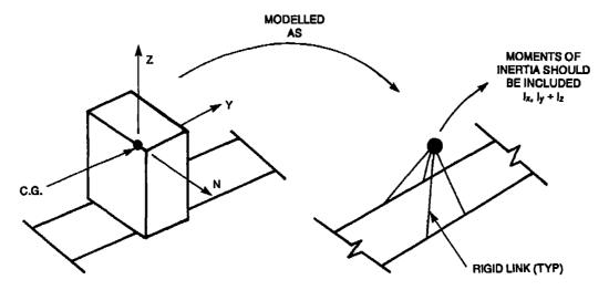
FIGURE 3-2.6 Modelling Rotational Inertia
