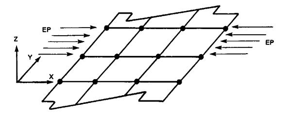
FIGURE 3-3.18 Definition of Edge Pressure
