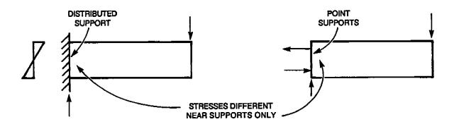
FIGURE 3-2.3 Illustration of St. Venant's Principle
