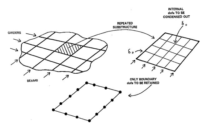
FIGURE 3-3.9 Schematic Illustration of The Static Condensation Process
