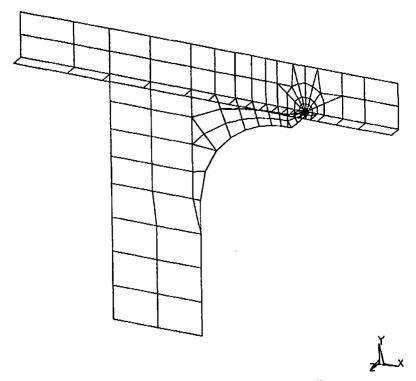
FIGURE 4.2-5 Benchmark Problem BM-5 : Bracket Detail
