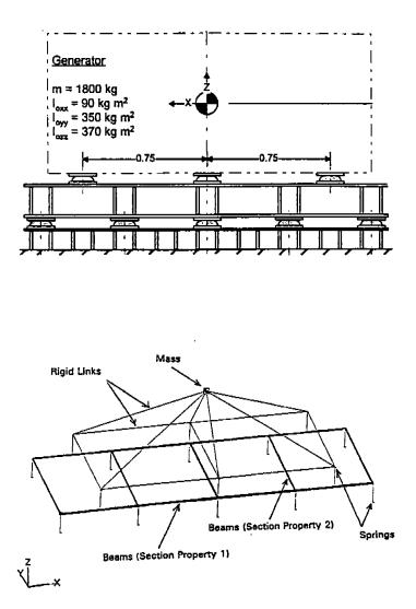
FIGURE 4.2-3 Benchmark Problem BM-3 : Vibration Isolation System
