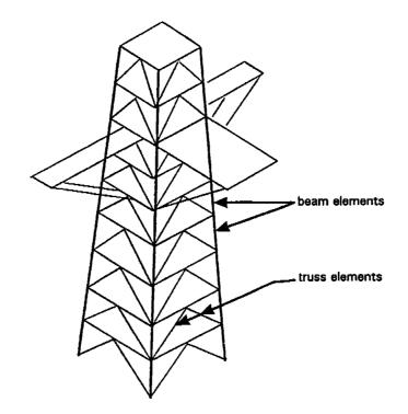
FIGURE 3-3.1 Typical Lattice Structure
