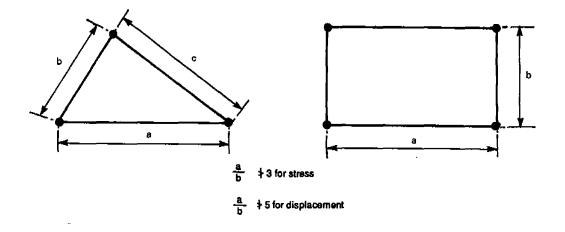
FIGURE 3-3.2 Aspect Ratio of Plane Elements
