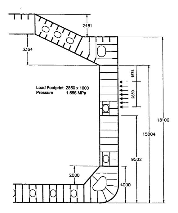
FIGURE 3.3 Characteristics of Load
