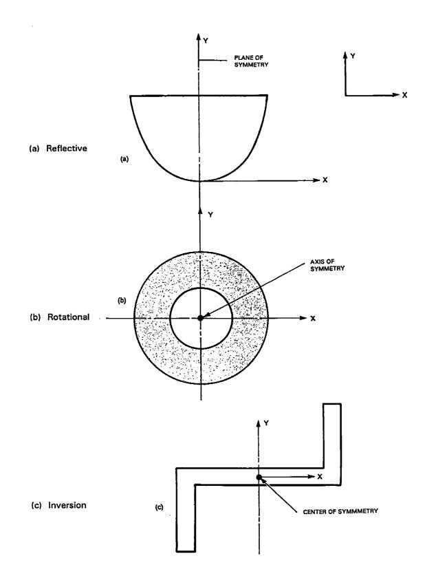
FIGURE 3-3.12 Different Types of Symmetry
