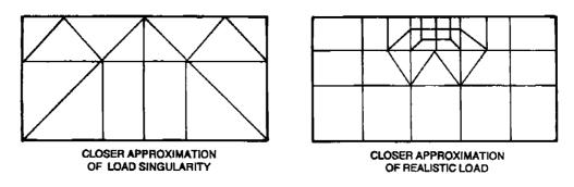
FIGURE 3-3.5 Transitions Using Triangular Elements
