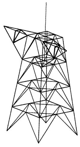
FIGURE 4.2-4 Benchmark Problem BM-4 : Mast Structure
