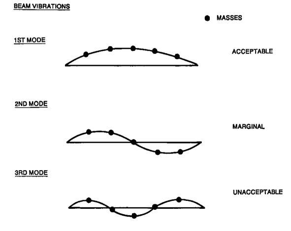
FIGURE 3-2.4 Mass Distribution Required for Accurate Determination of Natural Frequencies
