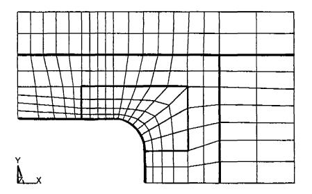
FIGURE 4.2-1 Benchmark Problem BM-1 : Reinforced Deck Opening
