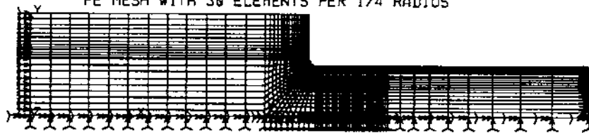
FE MESH WITH 30 ELEMENTS PER 1/4 RADIUS
