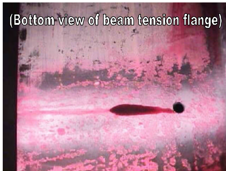
Figure 11-35: Enlarged hole captures the crack tip.
