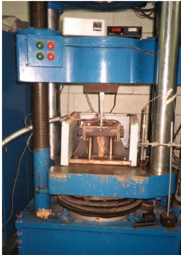
Figure 3.2: CCA test set up for specimen size W = 300 mm.
