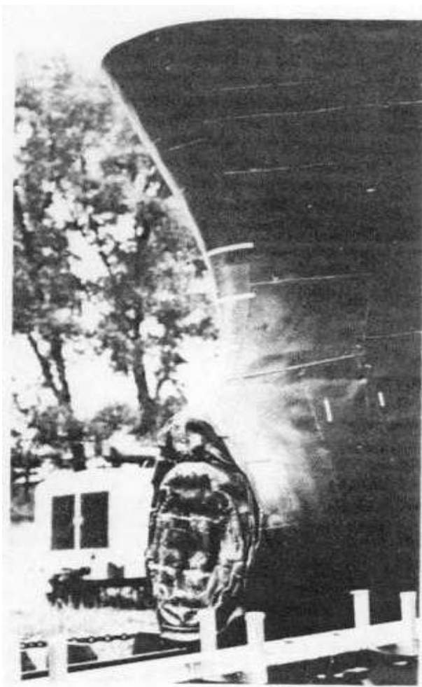
Figure 29 - Esso Malaysia Model after Damage [37]
