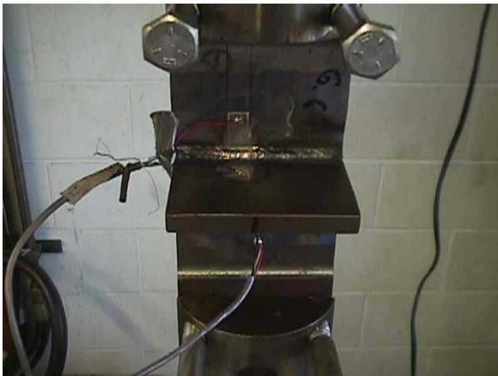
Figure 7.7(b): Photograph of the Cruciform Specimen in the Fatigue Testing Rig
