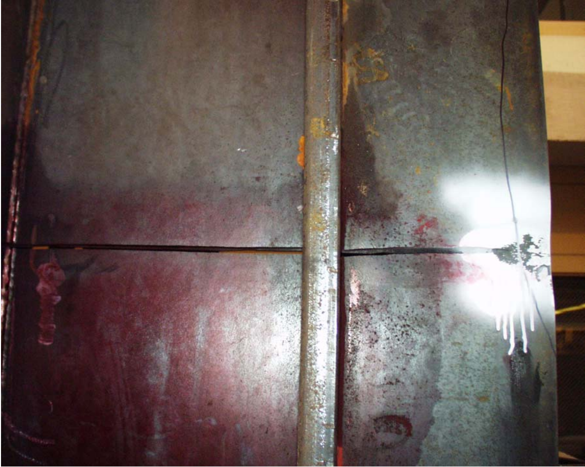
Figure 3-14 Plastic zone forming at the crack tip
