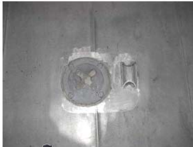
Figure 6-21. Typical Cloverleaf Tiedown Shown on HSV-X1 (With Original Tiedown Tube)
