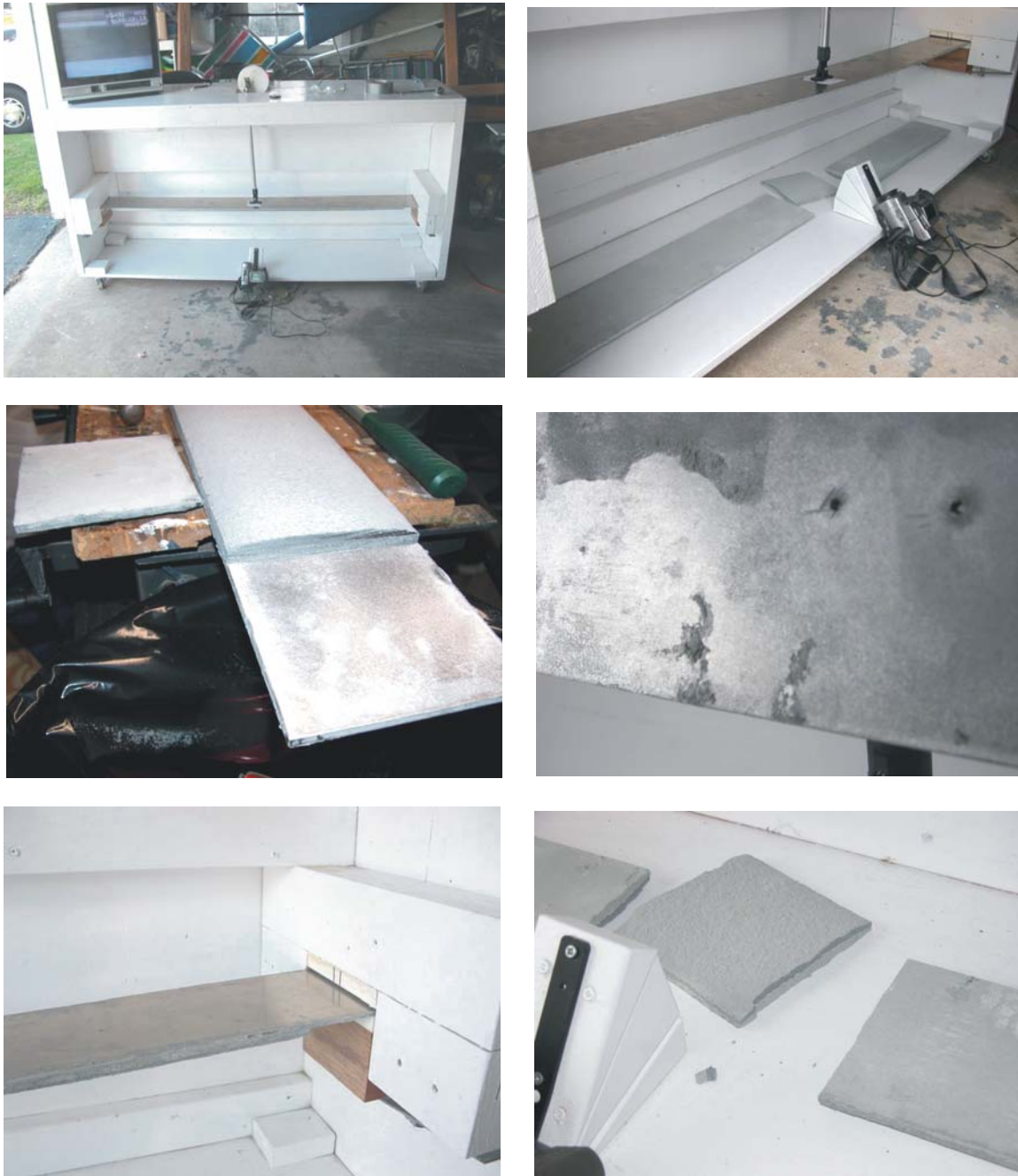
Figure 22 Photographs of Superior SP2001F Aluminum Panels. Photos at left show panels being prepared for testing and the start of the test. The photos at right show the failed coating on the aluminum panels and the surface of the aluminum panel.
