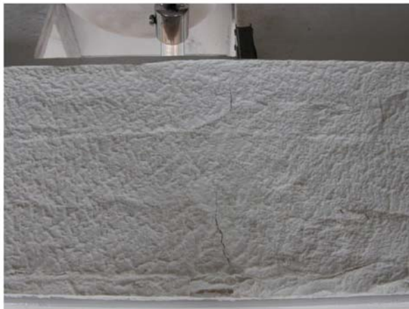
Figure 17 Preparation, Coating and Finished Coating Surface for Fyre Shield Product from CHI Technologies (note coating being “trowel applied” using built up dam)
