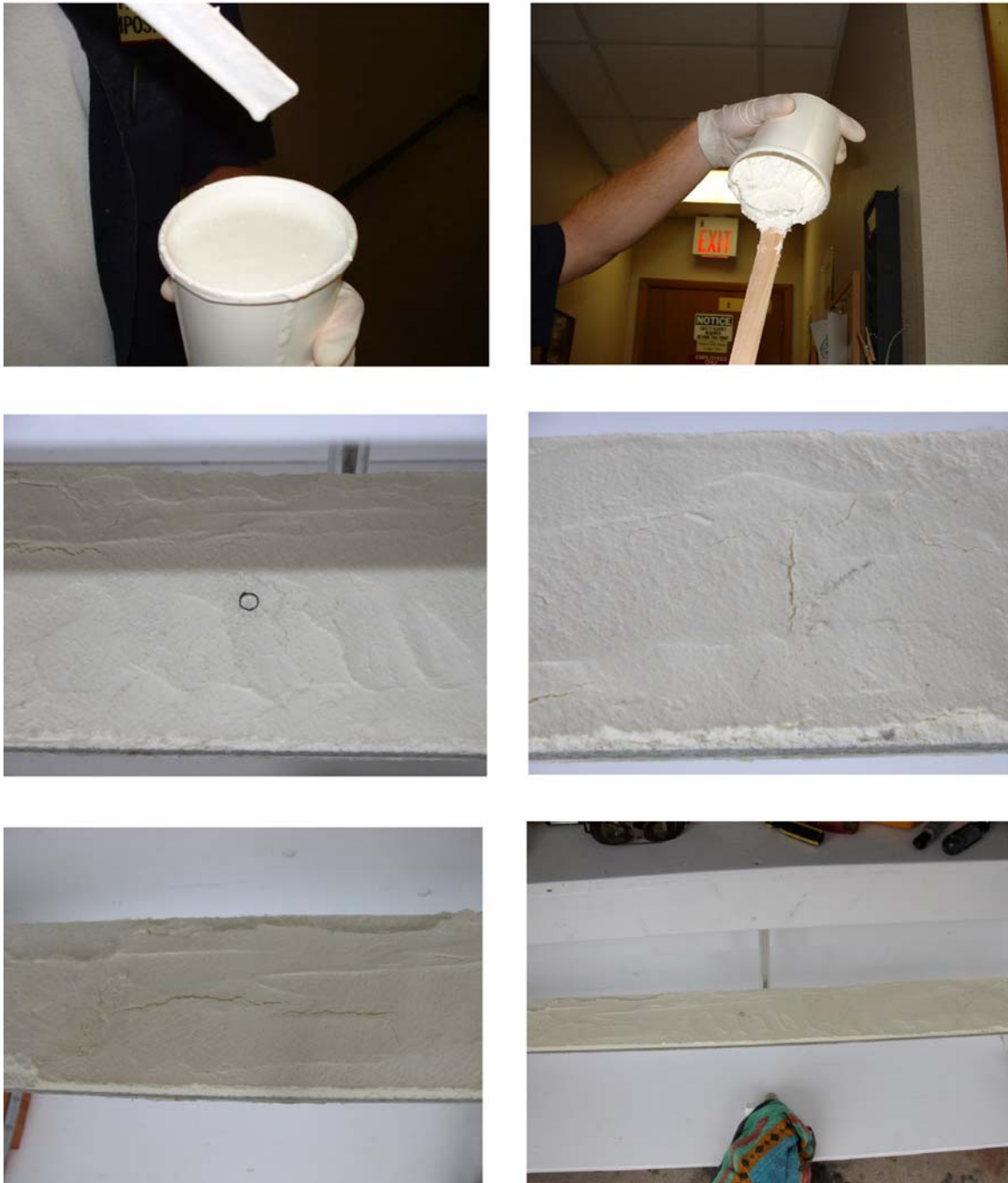
Figure 19 Photographs Showing Fastblock 810 in Liquid Form and after Cured in a Paint Bucket (top row) The Photos in the Middle Row Shows Area Where Mounting Screw Penetrates Coating Surface and Transverse Cracking Evident after Testing. The Bottom Row Shows Overall Surface Unevenness.
