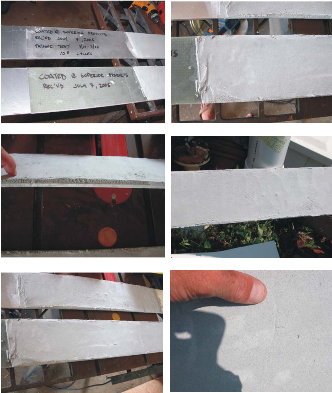
Figure 26 Pictures of SP2001F Retest (clockwise from top left) Panels Received July 7, 2005; Detail of Coating Edge Finish; Coating Thickness About Half of Original Panels; Coating Appearance After Impact Test; Aluminum and Composite Panels After Testing; and Detail of Tested Panel Showing Minor Surface Crack
