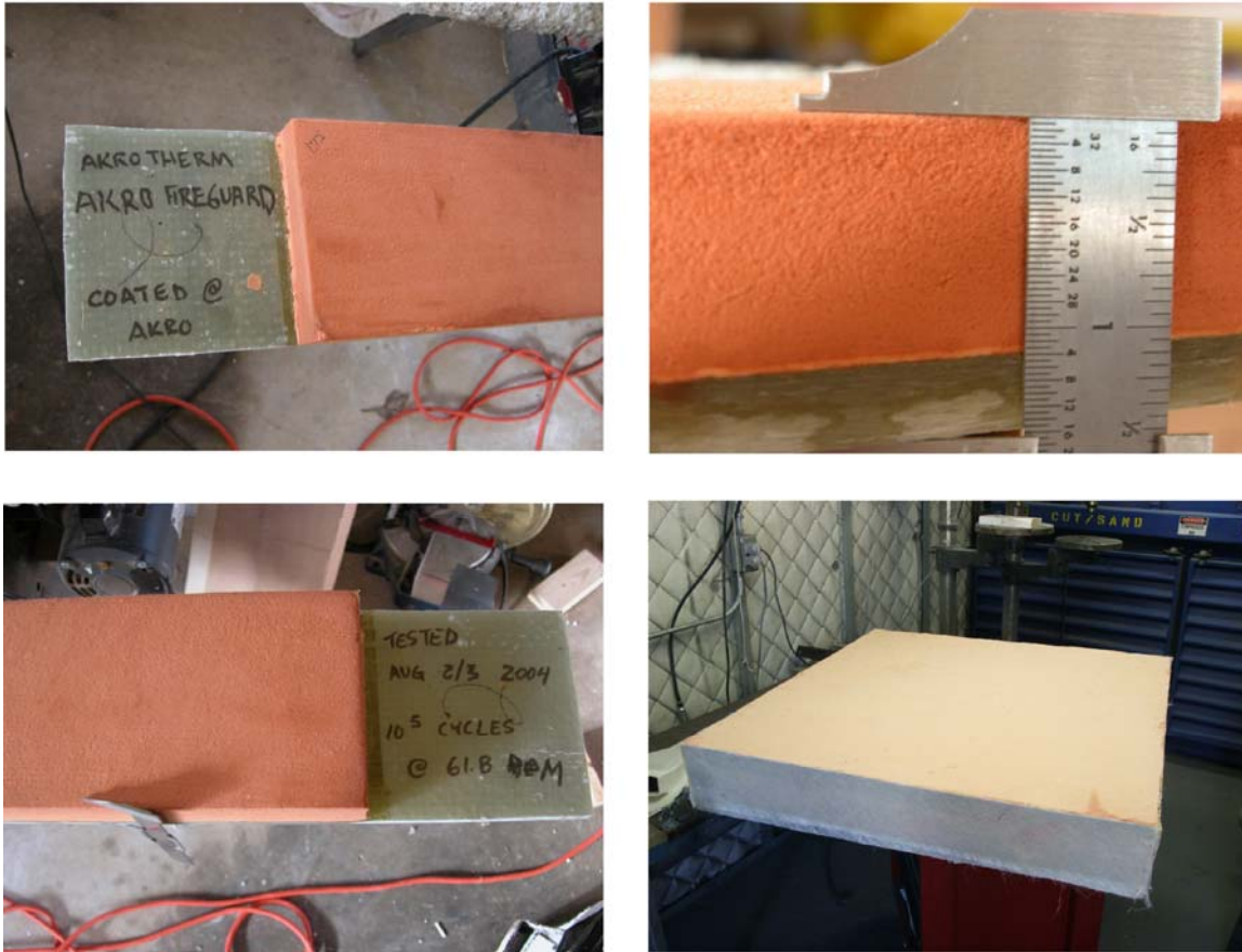
Figure 18 Photos of the Panel Coated with Akro Therm by Akro Fireguard. The Photograph in the Lower Right Shows a Test Panel that NGSS and Akro Fireguard Fire Tested using UL 1709 Fire Insult
