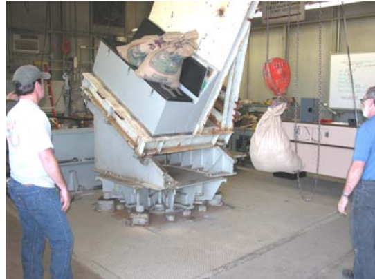
Figure 2 Seat Being Tested to MIL-STD 901D with 45° Test Fixture
