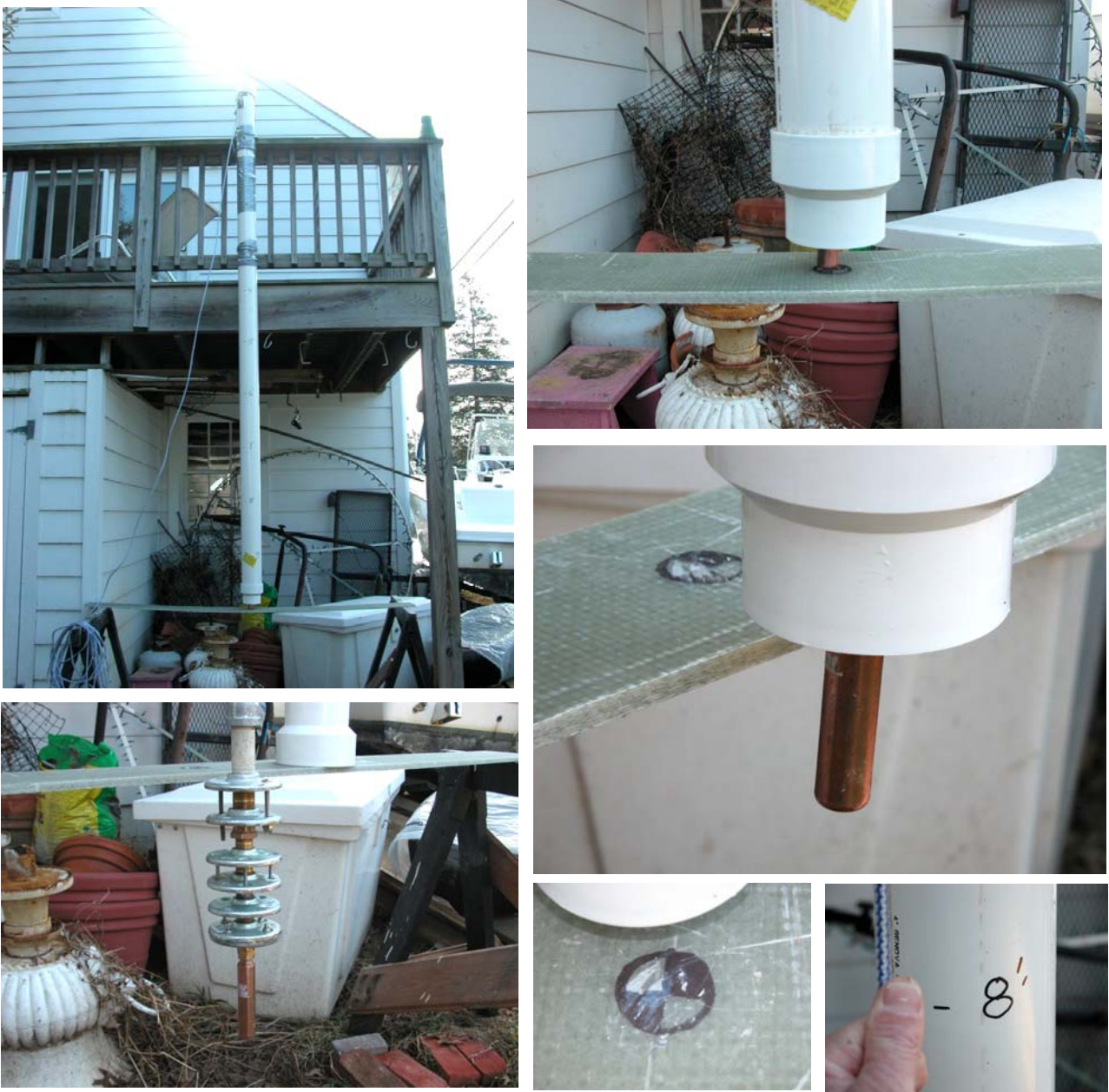
Figure 25 Pictures of Shock Test Arrangement (clockwise from top left) 10' Long PVC Tube Mounted to Elevated Deck; Impactor Relationship to Test Panel; Impactor Shown Fully Extended from Tube; Weight Raised 8 feet for Ten Impact Hits; Impact Effect on Composite Test Panel; and View of Impactor Assembly (6.25 pounds)
