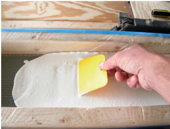
Figure 17 Preparation, Coating and Finished Coating Surface for Fyre Shield Product from CHI Technologies (note coating being “trowel applied” using built up dam)
