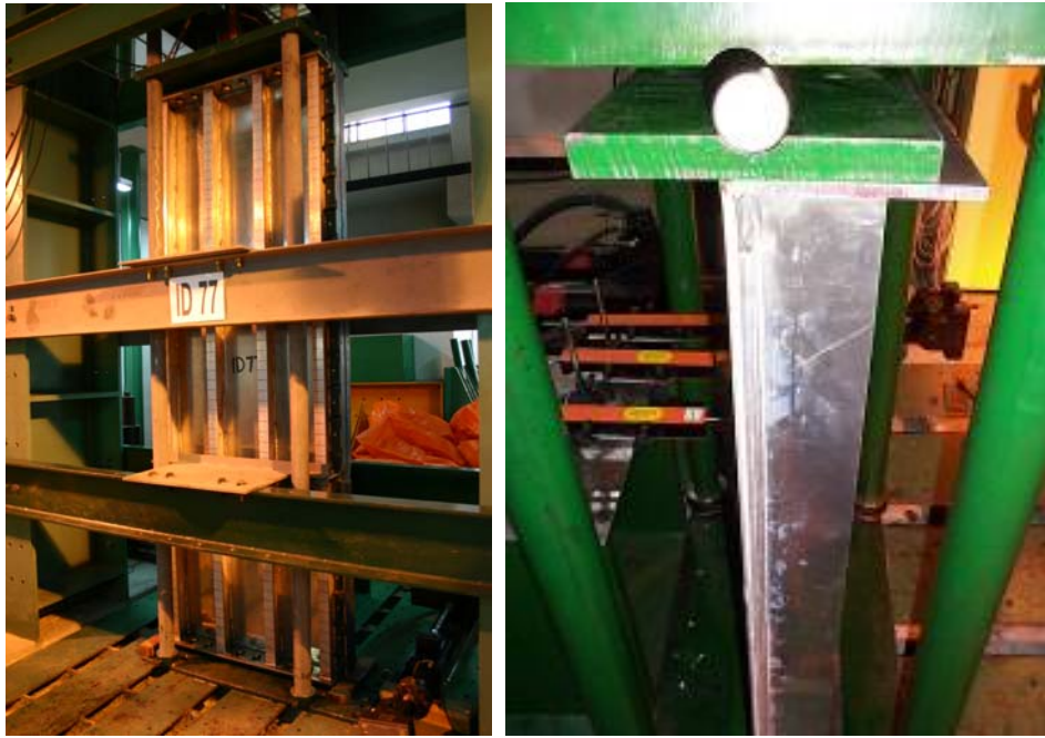
Figure 7.2 Simply supported condition at loaded edges and axial compressive loading at the neutral axis of the panel cross section
