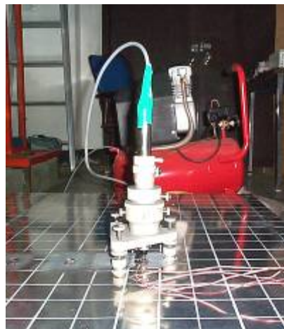
Figure 6.3 Hole drilling machine used for strain release measurement
