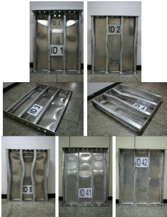
Figure 7.81 Selected photos of the test structures showing typical collapse modes (ID1: Mode III, ID2: Mode V, ID3: Mode III+IV, ID4: Mode IV+V, ID8: Mode V, ID41: Mode III, ID42: Mode IV)
