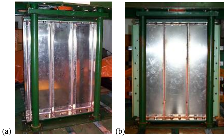
Figure 7.1 Test set-up for collapse testing on stiffened plate structures (a) without supporting jigs at unloaded edges, (b) with supporting jigs at unloaded edges to keep them straight
