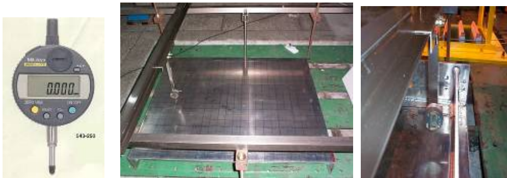
Figure 6.1 Dial gauge and its attachment for initial distortion measurement
