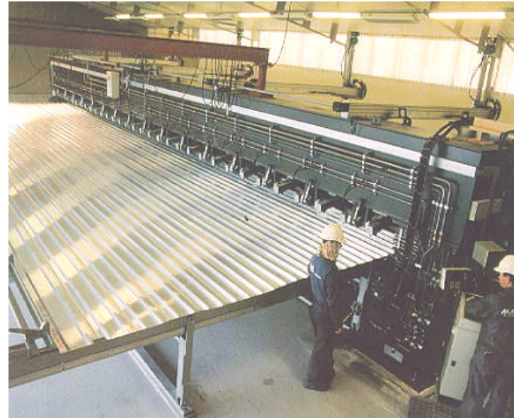
Friction stir welding panels together (Advanced Joining Technologies web site and The Welding Institute)
