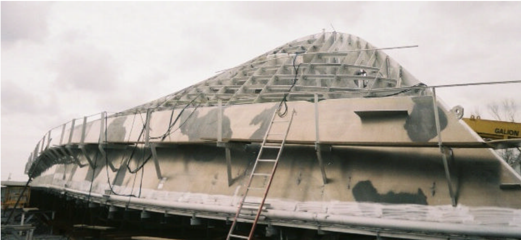
Hull with stick construction of framing (Courtesy of Gulf Craft)
