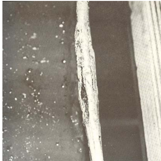
Example of exfoliation on the edge of a waterway bar (Dye and Dawson, 1974).
