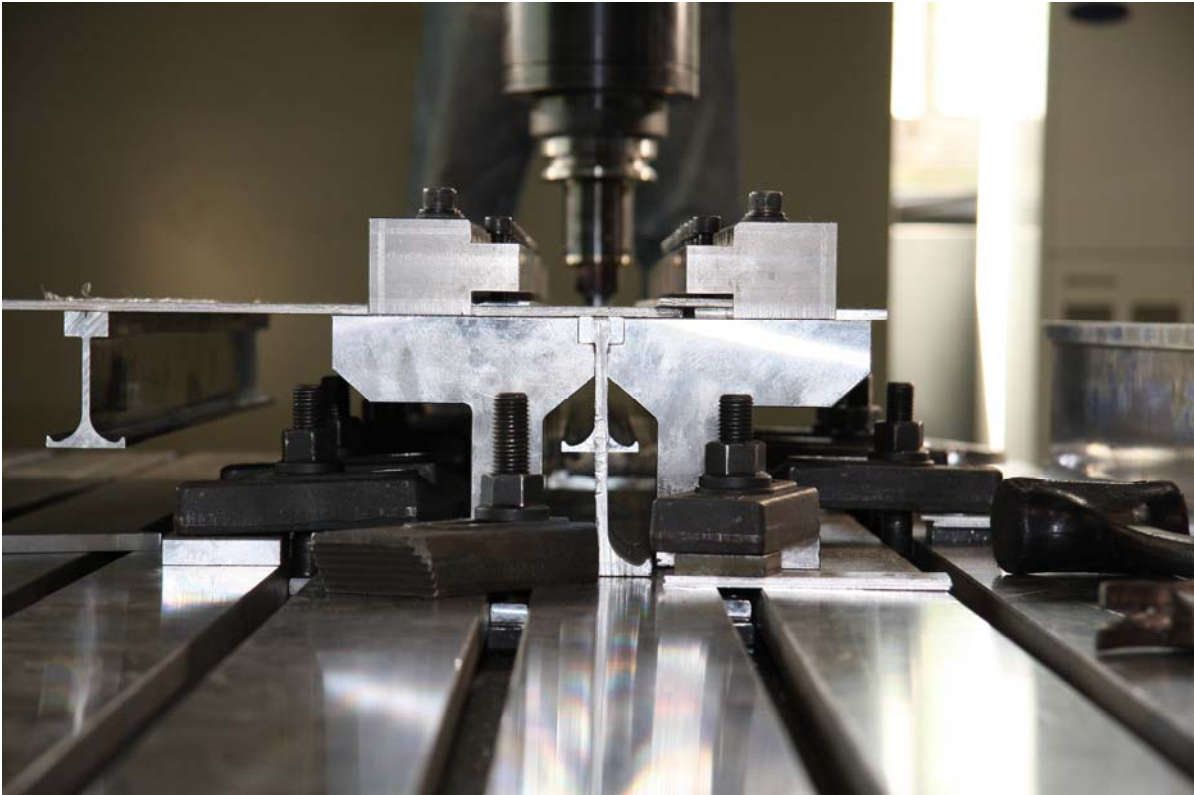
Figure 3.18(a) Photo of a test structure during friction stir lap-joining
