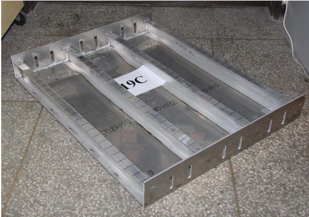
Figure 5.14(b) Photo of Collapse Mode II in test structure 19C
