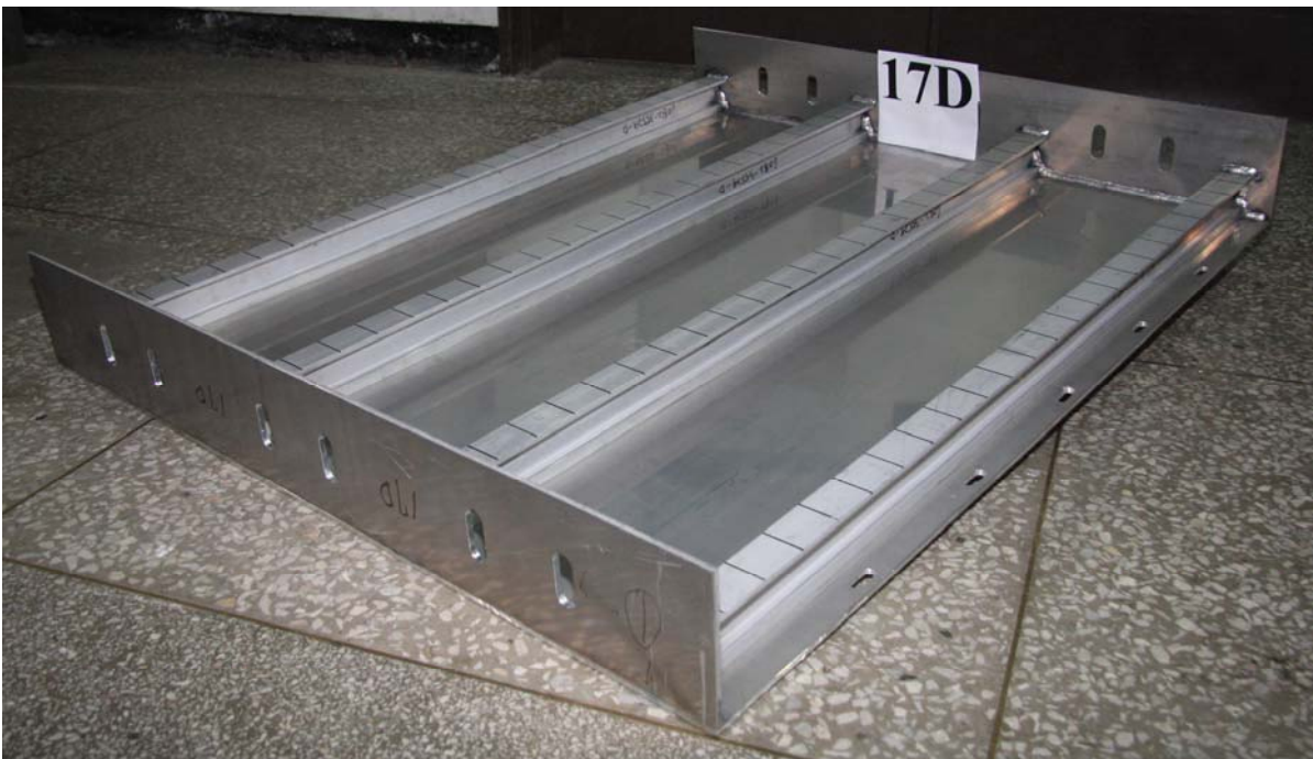
Figure 3.18(b) Photo of test structure 17D after friction stir lap-joining
