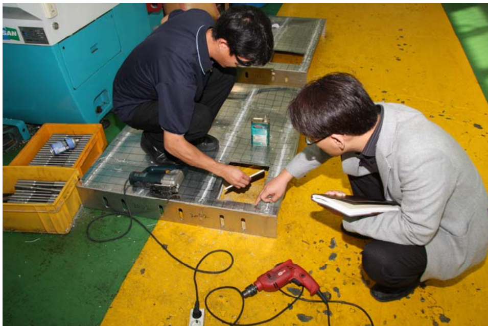
Figure A.11 Photo of one of the test structures after the material test specimen had been cut out of the buckling collapsed structure
