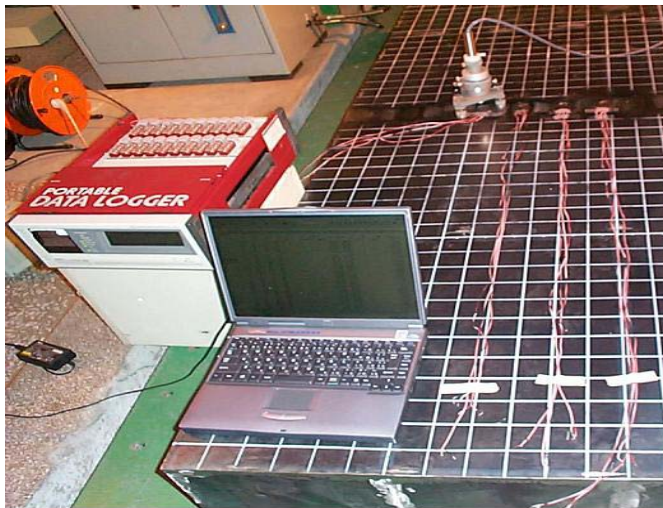
Figure 4.7 Set-up for residual stress measurement using the hole-drilling strain-gauge method
