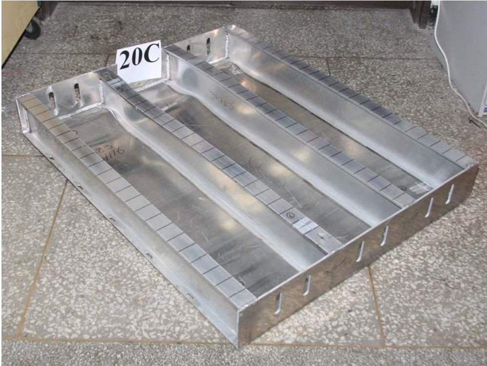
Figure 5.15(b) Photo of Collapse Mode IV in test structure 20C
