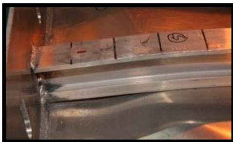
Figure 5.8(b) Photo of Collapse Mode III in test structure 17D
