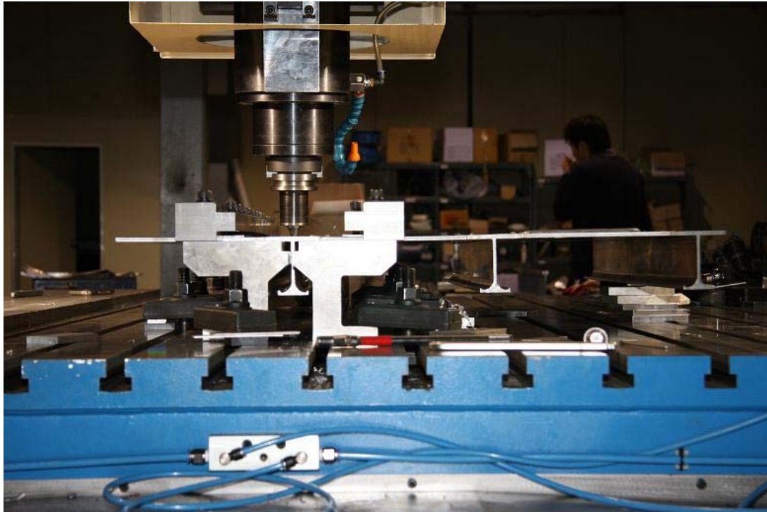
Figure 2.5 Photo of the FSW process applied for building the present test structures
