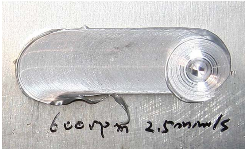
Figure 2.6 Keyhole at the end of the friction stir weld
