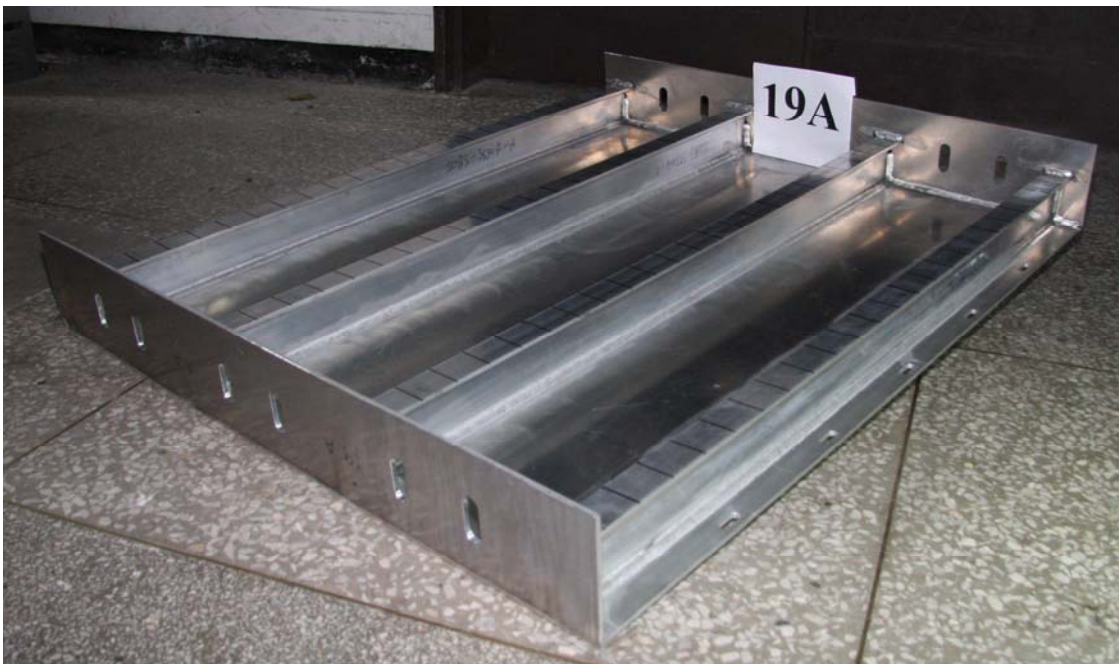
Figure 3.10(b) Photo of test structure (19A) after fusion-weld fabrication
