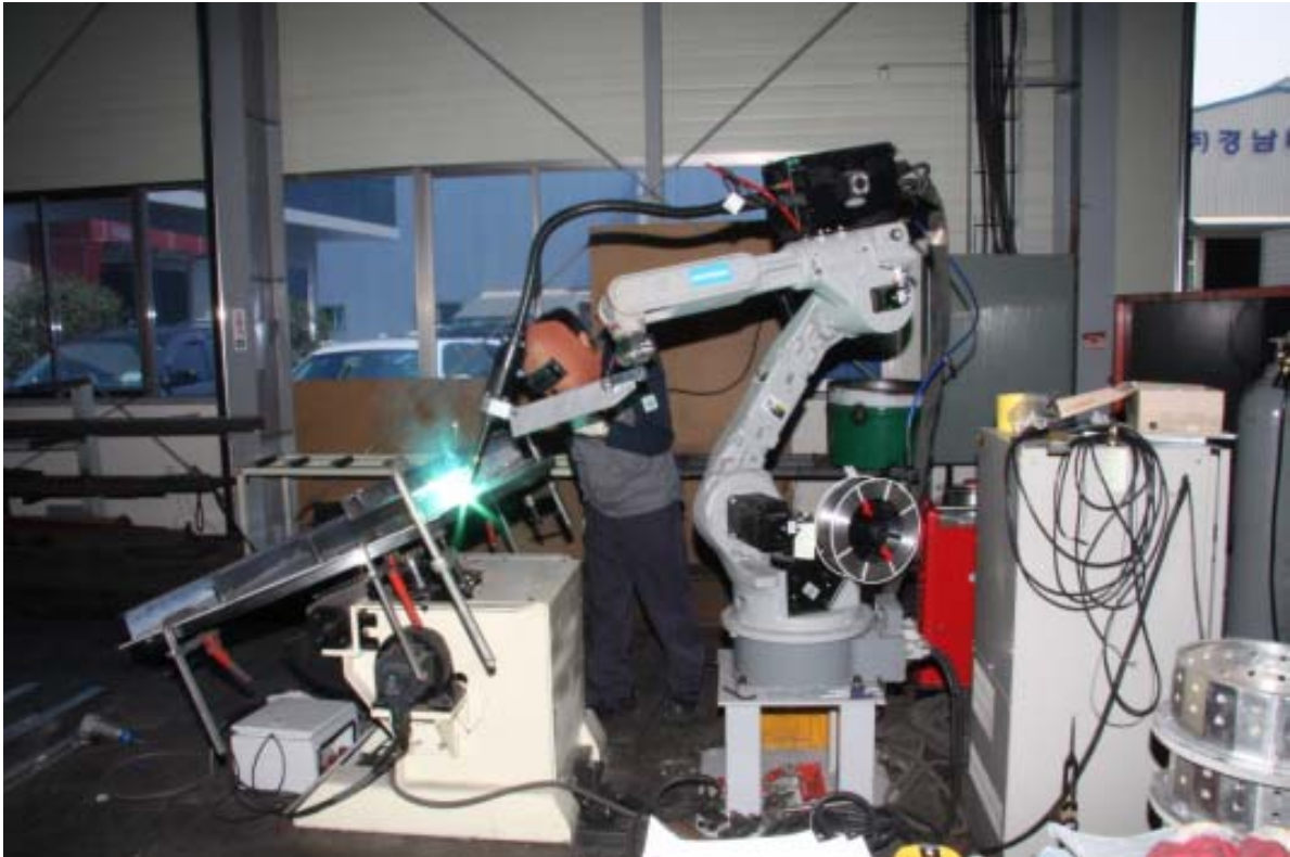
Figure 2.1 Photo of GMAW-based fusion-welding process applied for building the present test structures
