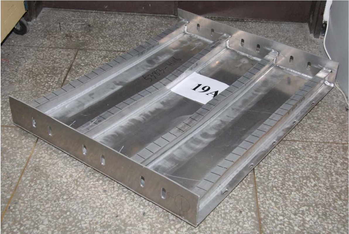
Figure 5.6(b) Photo of Collapse Mode V in test structure 19A
