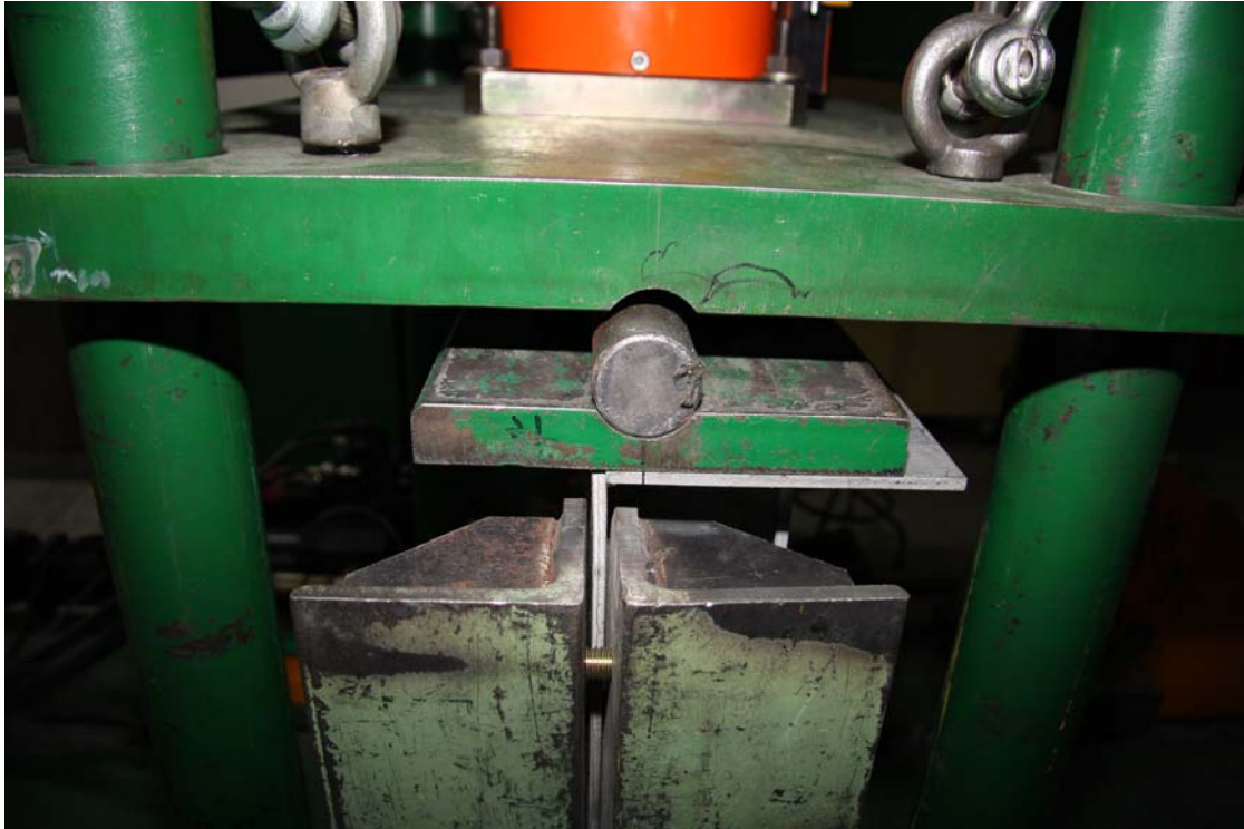
Figure 5.2 Photo of the rigid solid bar inserted into the loaded edge
