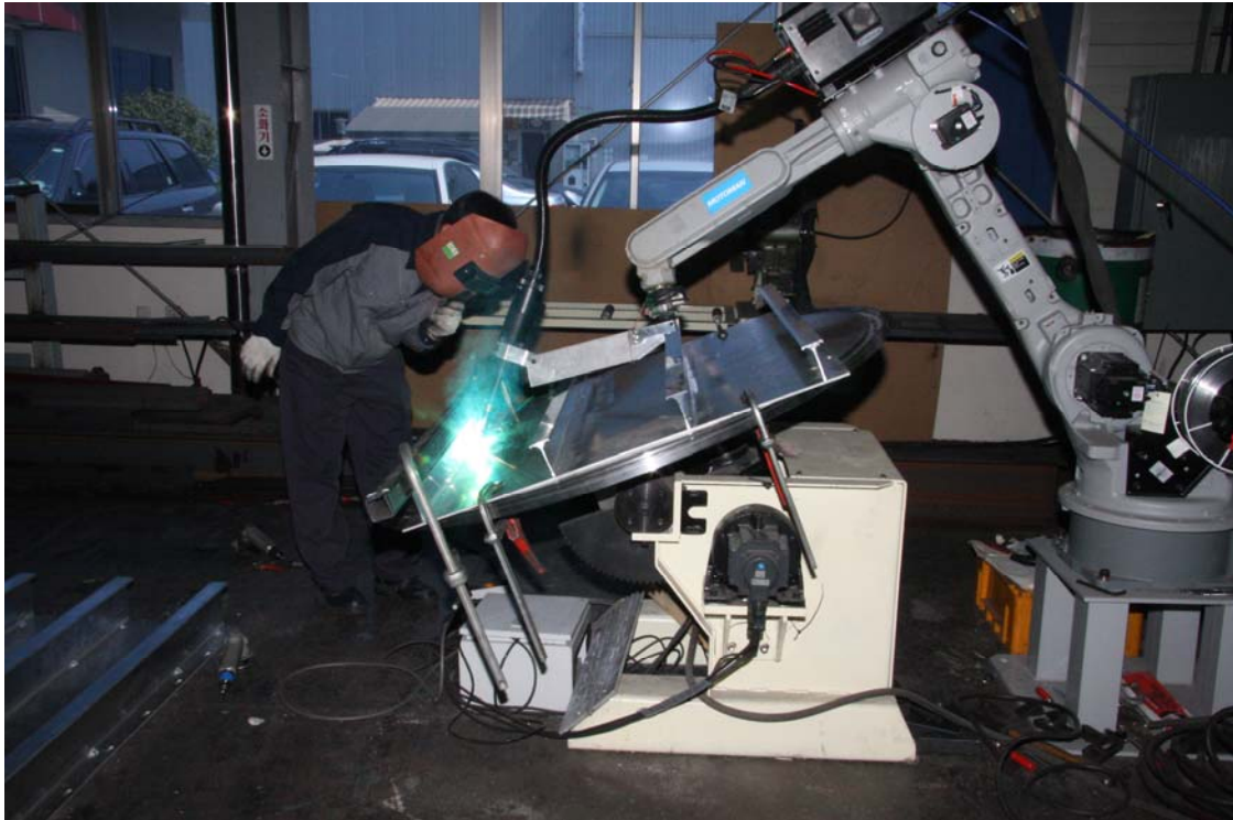
Figure 3.10(a) Photo of one of the test structures during fusion-weld fabrication
