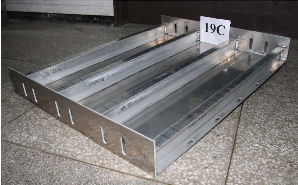
Figure 3.15(b) Photo of test structure 19C after friction stir butt-jointing
