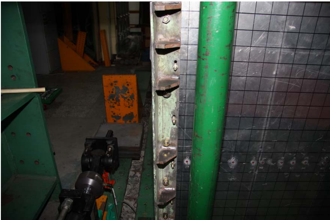
Figure 5.3 Photo of the rigid strips bolted to the test panel at the unloaded edge
