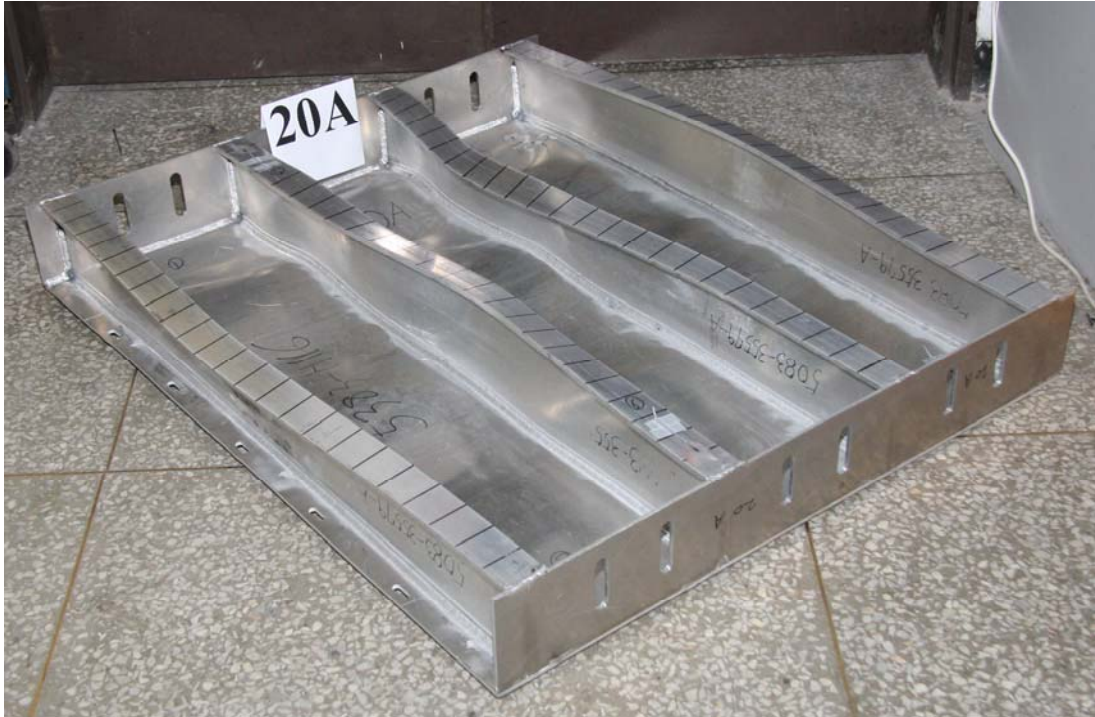
Figure 5.7(b) Photo of Collapse Mode IV in test structure 20A
