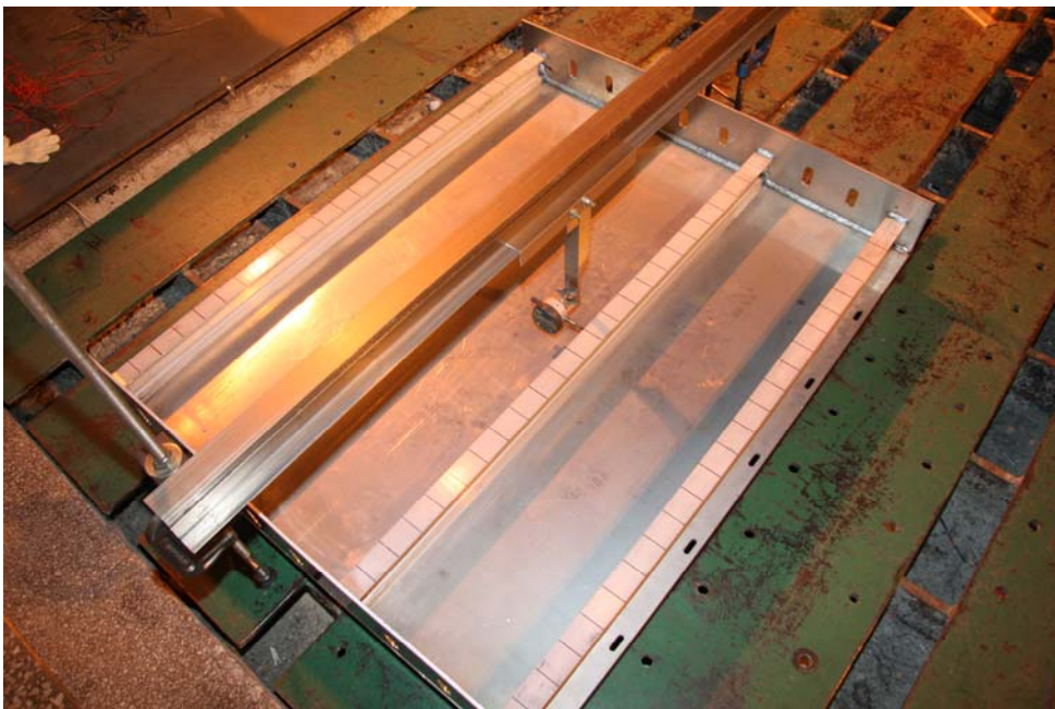
Figure 4.3(b) Photo of the set-up for the stiffener initial distortion measurements
