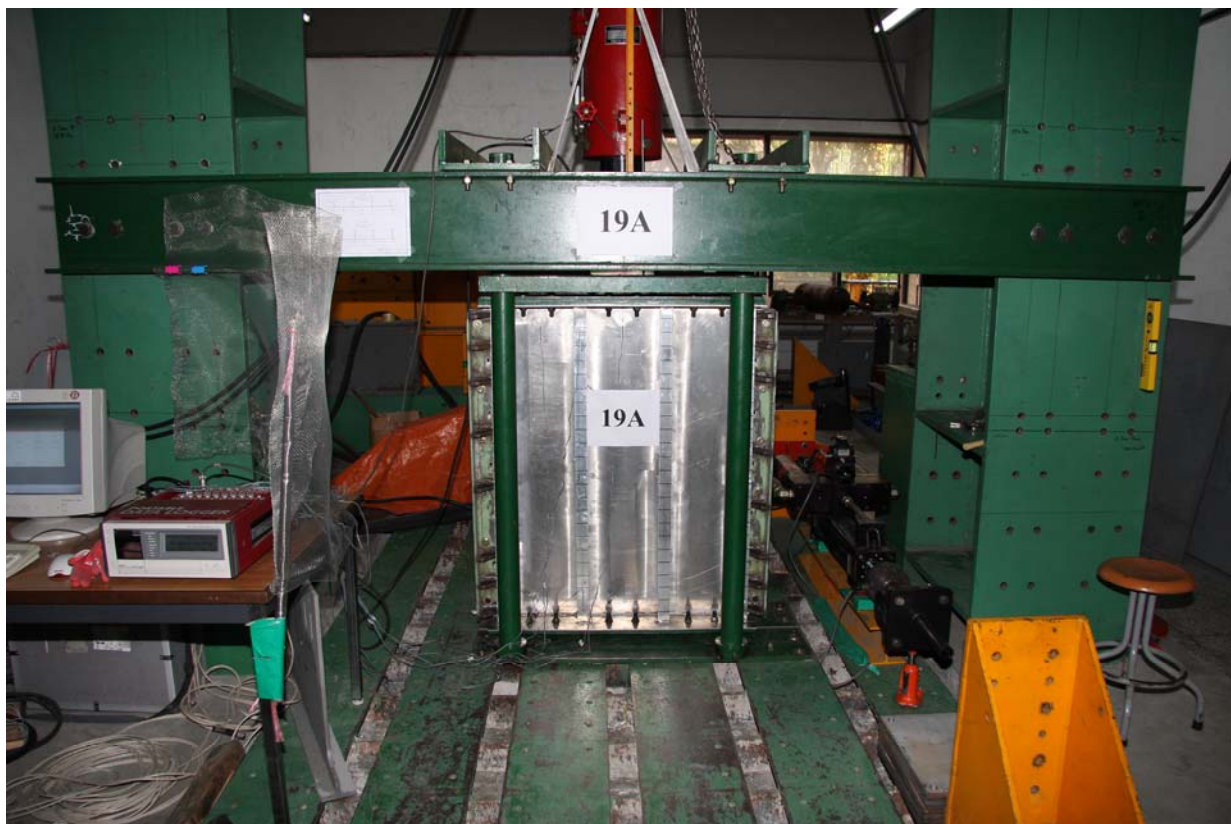
Figure 5.1 Photo of the test set-up for buckling collapse testing
