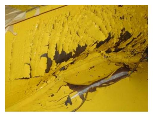
Figure 28: LG1\_2 test: close-up of web deformation at 330kips (1468 kN)
