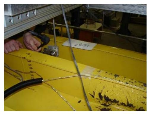
Figure 31: LG1\_3 at 198 kips (note: load is at center, with prior shear damage at end)
