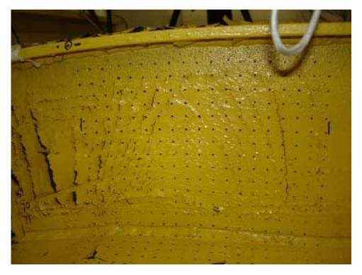
Figure 30: LG1\_2 test, web distortion
