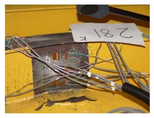
Figure 22: LG1\_1 test: web deformation at 281kips (1250 kN)
