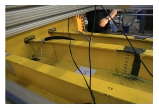
Figure 33: LG2\_2 at 202kips
