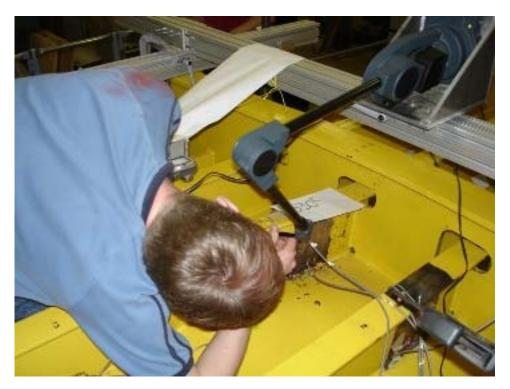
Figure 26: LG1\_2 test: MicroScribe measurements at 330 kips (1468 kN)
