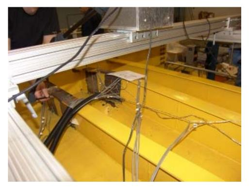
Figure 23: LG1\_1 test web deformation at 291kips (1294 kN)
