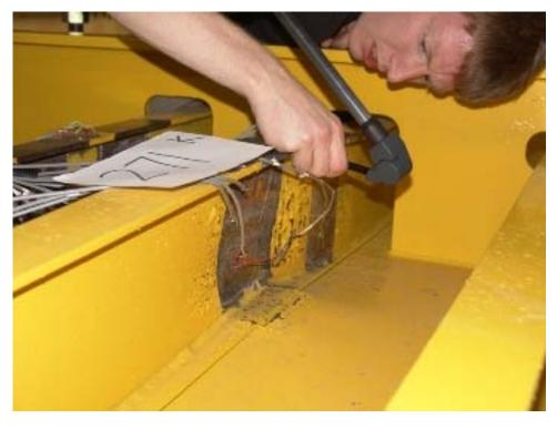
Figure 21: LG1\_1 test: MicroScribe measurements at 271kips (1205kN)
