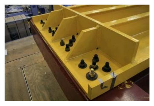
Figure 35: Large Grillage end clamp arrangement.
