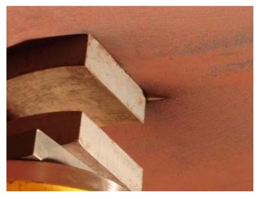
Figure 29: LG1\_2: ram after test (note imbedded platen and small tear)
