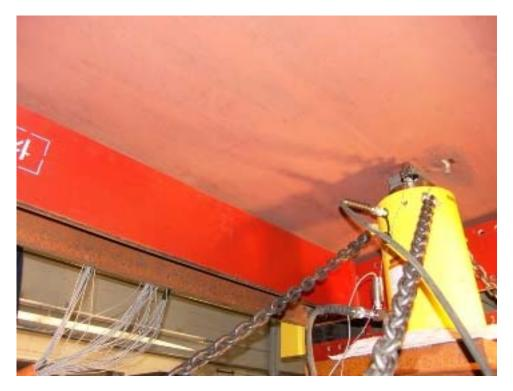
Figure 25: LG1\_1 view of ram after test (note imprint)
