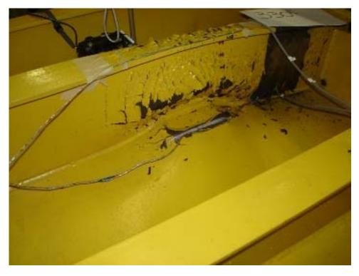
Figure 27: LG1\_2 test: web deformation at 330kips (1468 kN)
