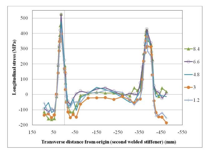
Figure 8.22: Longitudinal stress through the depth in the transverse (T) direction on line 1-2-3-4 (at L = 0 mm)
