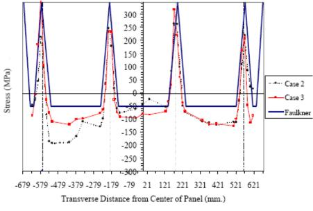
Figure 9.3: Faulkner residual stress model compared to measured values of two specimens (Dexter & Pilarski, 2000)
