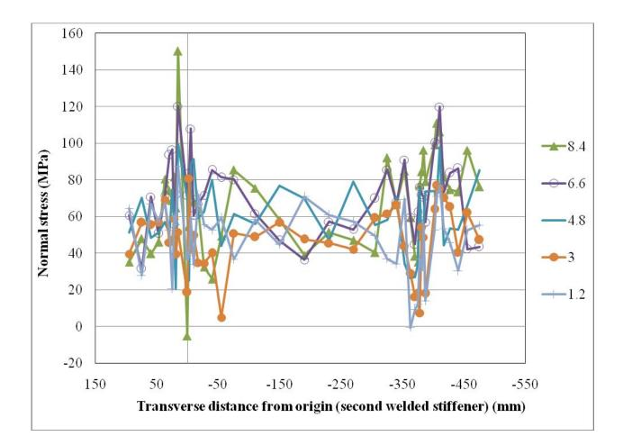
Figure 8.20: Normal stress through the depth in the transverse (T) direction on line 1-2-3-4 (at L = 0 mm)
