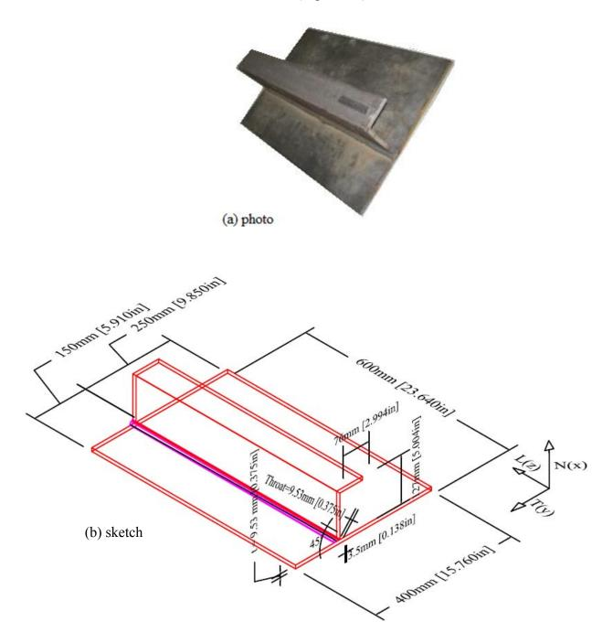
Figure 7.2: Specimen 2 (a) is a photo and (b) is the sketch
