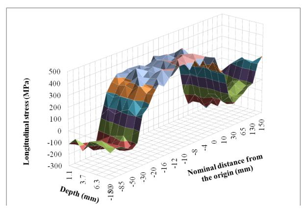
Figure 7.25: 3-D view of longitudinal stress distribution in transverse (T) direction (at L = 0 mm, line 3-1-4)
