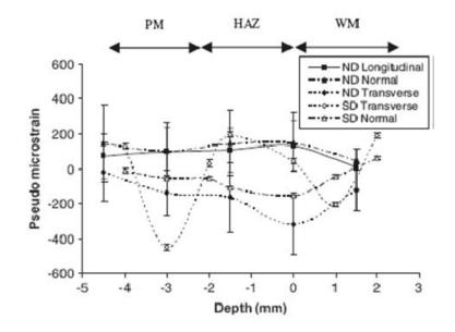
Figure 2.14: Pseudo-strain measured by ND and SD through the thickness (Paradowska, Finlayson, et al., 2006)
