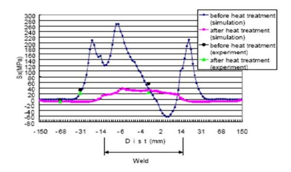
Figure 2.4: Comparison of experimental and simulation residual stresses (Cho, et al., 2004)
