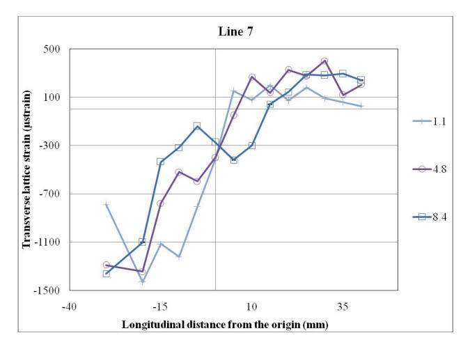
Figure 8.12: Transverse strain at various depths in the longitudinal (L) direction on line 7 (at T = 10 mm)
