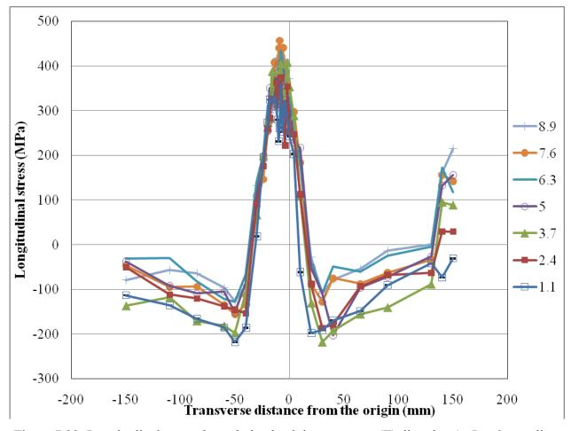
Figure 7.23: Longitudinal stress through the depth in transverse (T) direction (at L = 0 mm, line 3-1-4)
