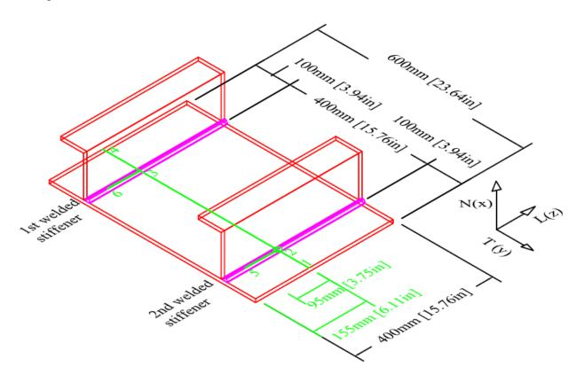
Figure 8.18: Detail for Measurement Points for Specimen 5
