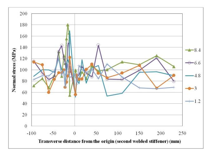
Figure 8.27: Normal stress at various depths in the transverse (T) direction on line 1-2-3 (at L = 0 mm)
