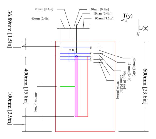
Figure 8.3: Detail for Measurement Points for Specimen 4
