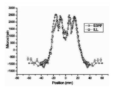
Figure 2.22: Centerline longitudinal strain measured in the two as-welded 12-mm-thick plates using neutrons and synchrotron X-rays (Ganguly, Fitzpatrick, & Edwards, 2006)
