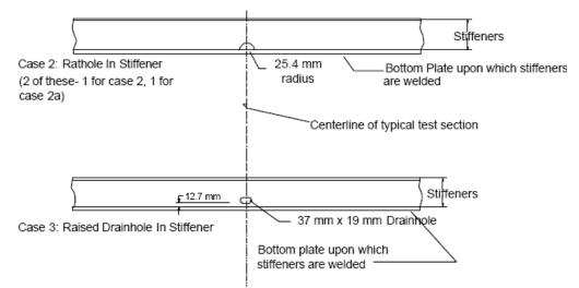
Figure 9.1: Specimen Details (Dexter & Pilarski, 2000)
