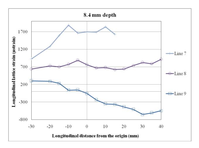
Figure 8.17: Longitudinal strain at a depth of 8.4 mm in the longitudinal (L) direction on lines 7, 8, and 9
