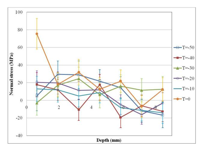
Figure 7.5: Normal stresses through the depth in transverse (T) direction (line 1-2)
