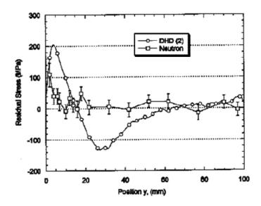
Figure 2.17: Longitudinal stresses in the 100 mm T-plate obtained by ND on a 12.5 mm slice and by DHD (Wimpory, et al., 2003)
