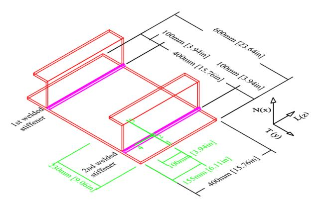
Figure 8.25: Details for Measurement Points for Specimen 6
