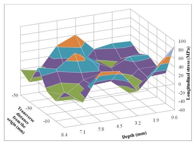
Figure 7.15: 3-D view of transverse stress distribution in transverse (T) direction (line 1-2)
