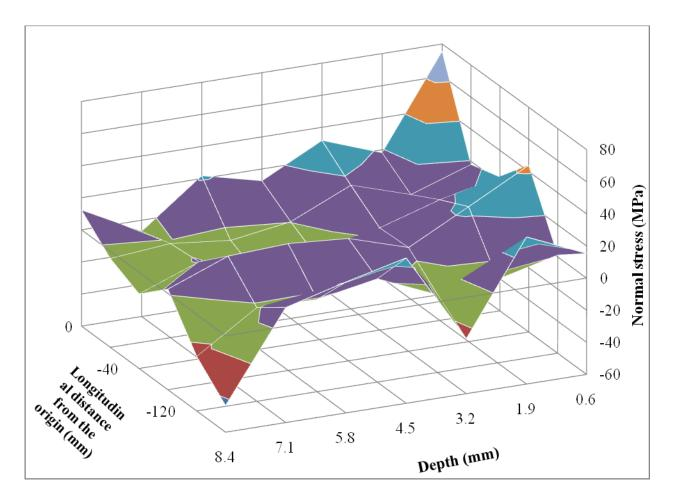
Figure 7.8: 3-D view of normal stress distribution in longitudinal (L) direction
