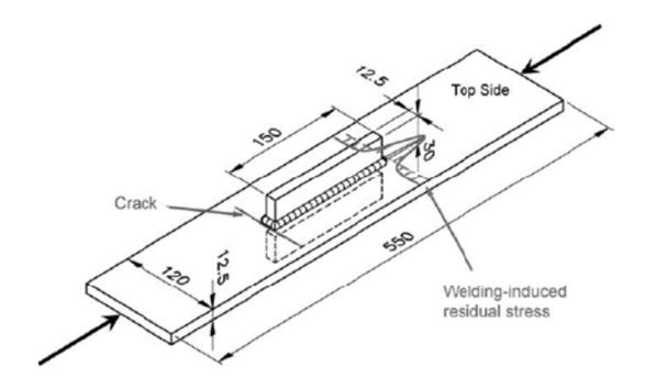
Figure 2.7: Test specimen with a typical crack and residual stress distribution (Rörup, 2005)
