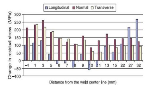
Figure 2.20: Change in stress in fully restrained sample in comparison to unrestrained sample (Price, et al., 2006)
