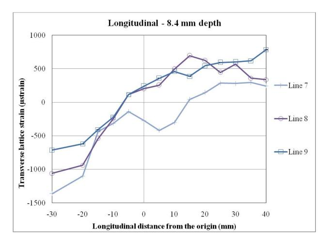
Figure 8.15: Transverse strain at a depth of 8.4 mm in the longitudinal (L) direction on lines 7, 8, and 9
