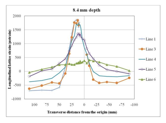
Figure 8.16: Longitudinal strain at a depth of 8.4 mm in the transverse (T) direction on lines 1, 3, 4, 5, and 6
