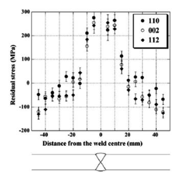
Figure 2.21: Longitudinal stress derived from measurements of {110}, {002} and {112} reflections in the high strength steel SNC631 as a function of position through the weld (Holden, Suzuki, et al., 2006)
