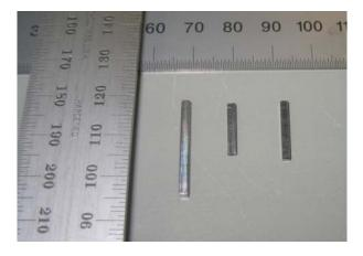
Figure 6.4: Stress-free reference samples
