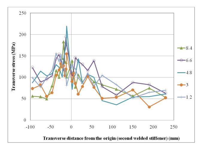
Figure 8.29: Transverse stress at various depths in the transverse (T) direction on line 1-2-3 (at L = 0 mm)
