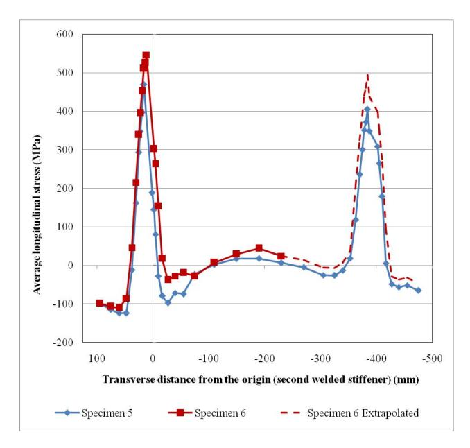
Figure 8.32: Average longitudinal stress distributions along the transverse lines (line 1-2-3-4 for Specimen 5 and line 1-2-3 for Specimen 6)
