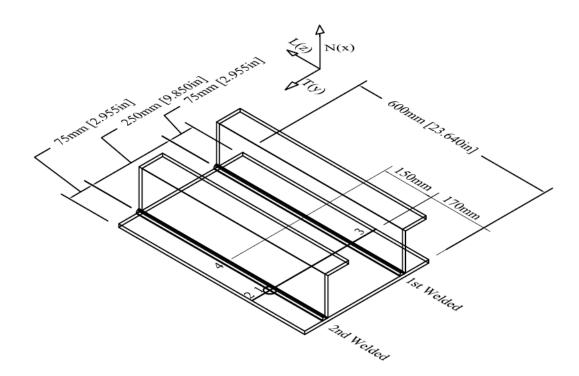
Figure 7.28: Detail for Measurement Points in Specimen 3
