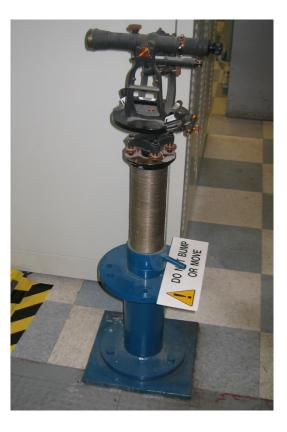
Figure 6.2: Level telescope pointed at the x-centre of rotation of the specimen
