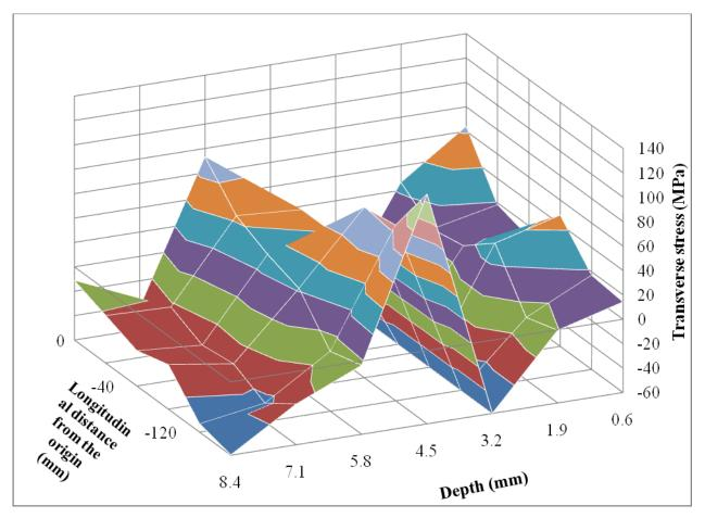
Figure 7.12: 3-D view of transverse stress distribution in longitudinal (L) direction (line 1-3)
