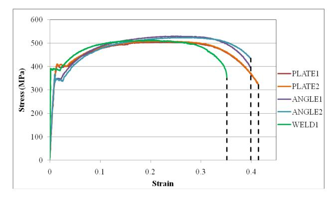
Figure 5.1: Nominal Stress-Strain Behaviour of Plate and Angle
