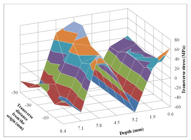
Figure 7.11: 3-D view of transverse stress distribution in transverse (T) direction (line 1-2)
