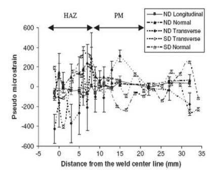
Figure 2.13: Pseudo-strain measured by ND and SD across the weld, (PM = parent material, HAZ = heat affected zone, WM, weld material) (Paradowska, Finlayson, et al., 2006)
