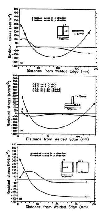
Figure 2.5: Residual stresses in welded specimens (Weng & Lo, 1992)
