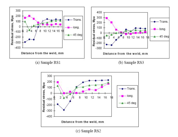
Figure 2.6: Surface residual stress distributions of (a) RS1 - 14kJ/cm, no restraint, (b) RS2 - 14kJ/cm, with restraint, (c) RS3 - 17kJ/cm, no restraint (Gao, et al., 1997)
