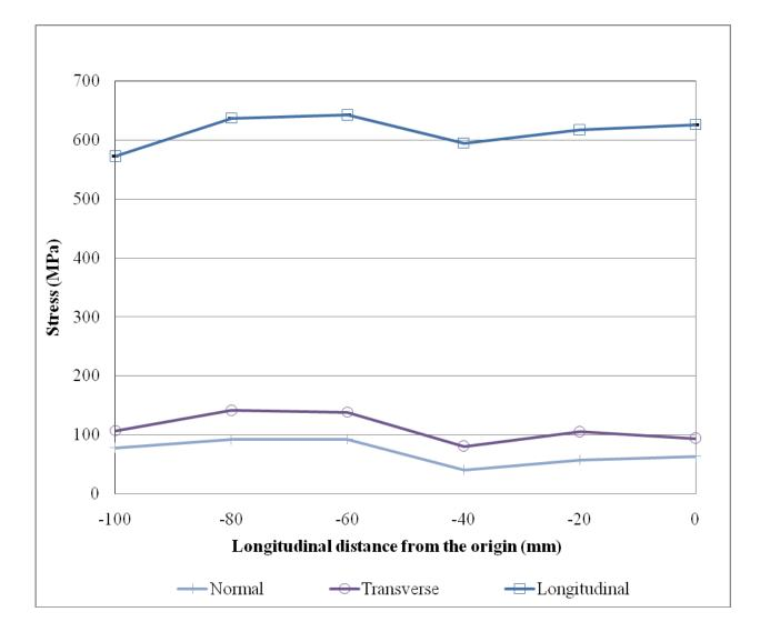
maximum difference of  $\pm 50$  MPa only indicating that the weld was uniform and consistent nature.
