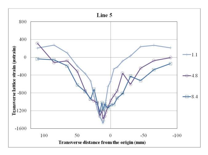
Figure 8.9: Transverse strain at various depths in the transverse (T) direction on line 5 (at L = -20 mm)
