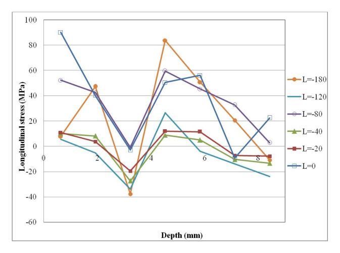
Figure 7.14: Longitudinal stress through depth in longitudinal (L) direction (line 1-3)
