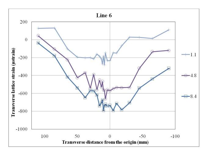
Figure 8.10: Transverse strain at various depths in the transverse (T) direction on line 6 (at L = -60 mm)
