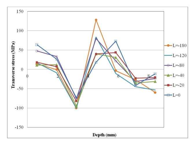
Figure 7.10: Transverse stress through the depth in longitudinal (L) direction (line 1-3)
