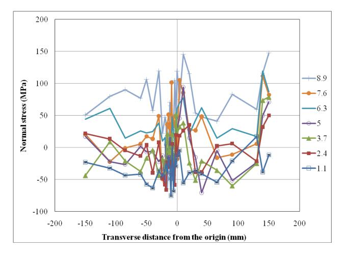
Figure 7.19: Normal stresses through the depth in transverse (T) direction (at L = 0 mm, line 3-1-4)
