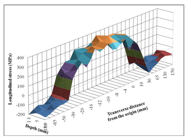
Figure 7.26: 3-D view of longitudinal stress distribution in transverse (T) direction (at L = 133 mm, line 5-2-6)
