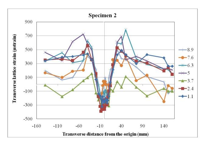
Figure 8.6: Transverse strain at various depths in the transverse (T) direction on line 1 (at L = 200 mm)
