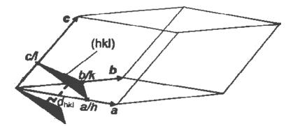
Figure 2.10: Lattice planes (Hutchings, et al., 2005)
