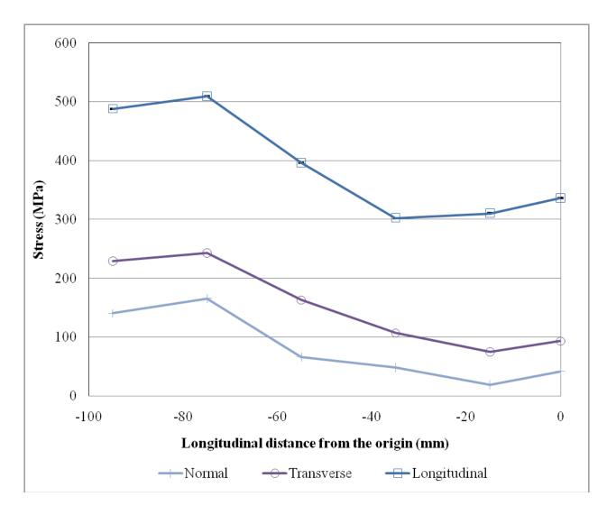
Figure 8.23: All stresses at first welded stiffener, at T = -390 mm, at N = 8.4 mm (on line 3-6)
