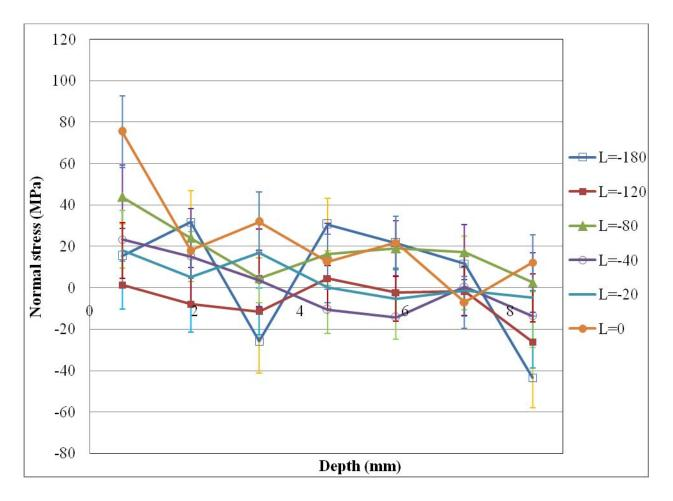
Figure 7.6: Normal stresses through the depth in longitudinal (L) direction (line 1-3)
