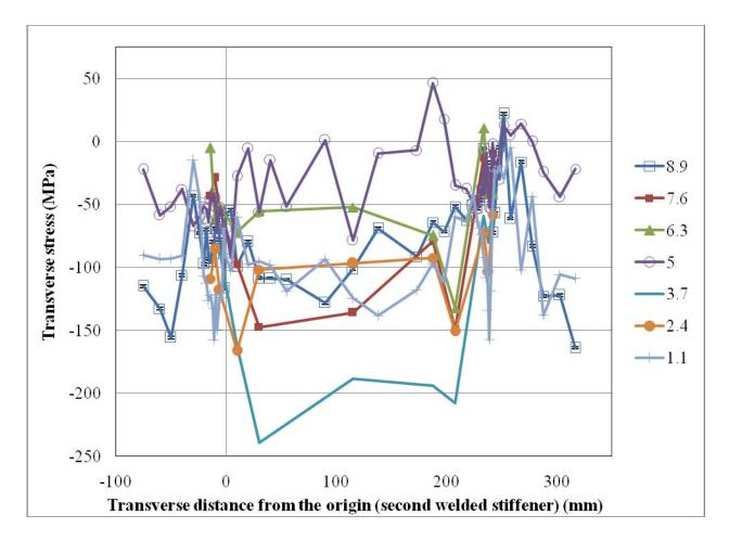
Figure 7.31: Transverse stresses though the depth in transverse (T) direction (line 2-1-3)
