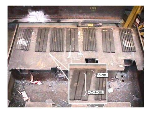
Figure 9.2: Sectioning coupons used for measuring residual stress distributions (Dexter & Pilarski, 2000)
