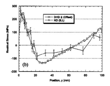
Figure 2.16: Transverse stresses in the 100 mm T-plate - ND measurement on a 12.5 mm slice and DHD measurement (Wimpory, et al., 2003)
