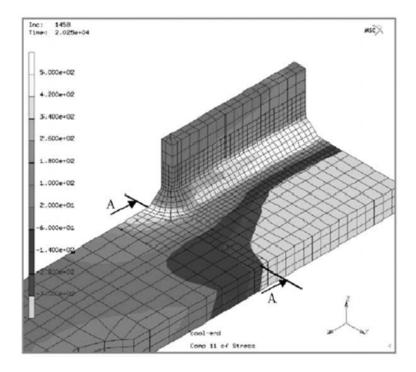
Figure 2.8: Analysis of the weld-induced residual stresses in the longitudinal direction (Rörup, 2005)
