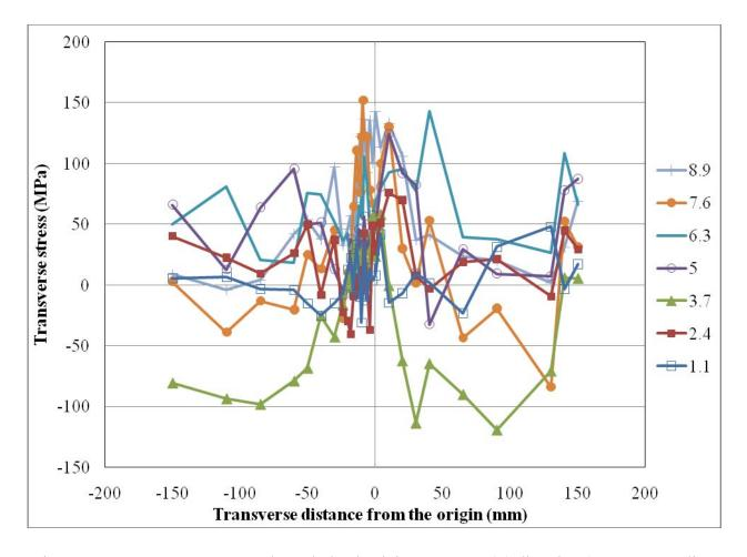
Figure 7.21: Transverse stresses through the depth in transverse (T) direction (at L = 0 mm, line 3-1-4)
