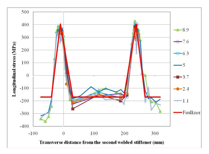
Figure 9.5: Specimen 3, two stiffeners spaced at 250 mm, high heat input
