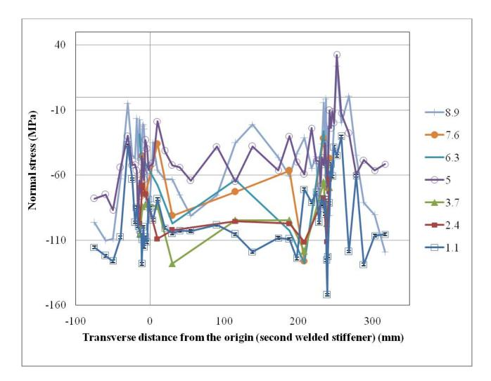
Figure 7.30: Normal stresses through the depth in transverse (T) direction (line 2-1-3)
