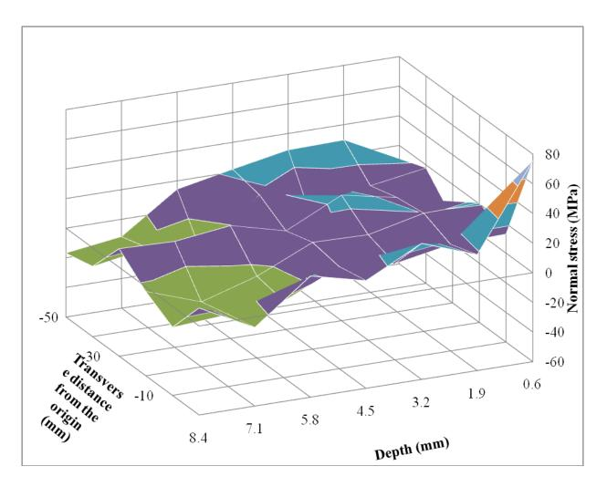
Figure 7.7: 3-D view of normal stress distribution in transverse (T) direction
