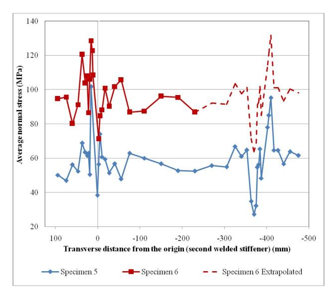
Figure 8.28: Average normal stress distributions along the transverse lines (line 1-2-3-4 for Specimen 5 and line 1-2-3 for Specimen 6)
