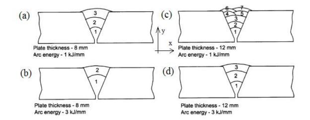
Figure 2.11: Cross-sectional details of the multipass weld runs used to make the butt joints in the 8mm and 12mm thick plates of RQT701 steel - (a) 8 mm plate thickness with low heat input (1 kJ/mm), (b) 8 mm plate thickness with high heat input (3 kJ/mm), (c) 12 mm plate thickness with low heat input, & (d) 12 mm plate thickness with high heat input (James, et al., 2006)
