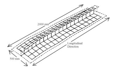
Figure 2.1: FE representation of the specimens (Hu & Jiang, 1998)
