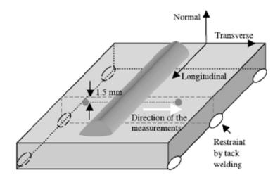
Figure 2.19: The direction of the measurements (transverse x, normal y, longitudinal would be z) using neutron diffraction on the single bead-on-plate (Price, et al., 2006)
