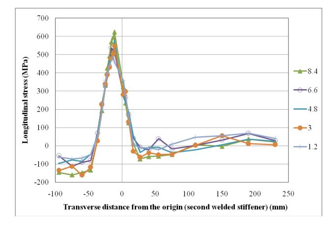
Figure 8.31: Longitudinal stress at various depths in the transverse (T) direction on line 1-2-3 (at L = 0 mm)
