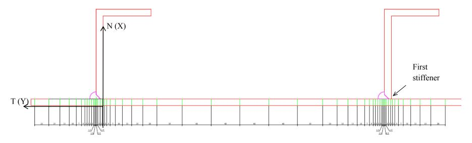
Figure 8.19: Spacing of the transverse direction measurements (in mm) on Specimen 5 (line 1-2-3-4)
