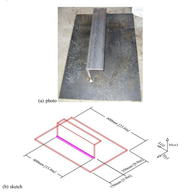
Figure 8.1: Specimen 4 (a) is a photo and (b) is the sketch
