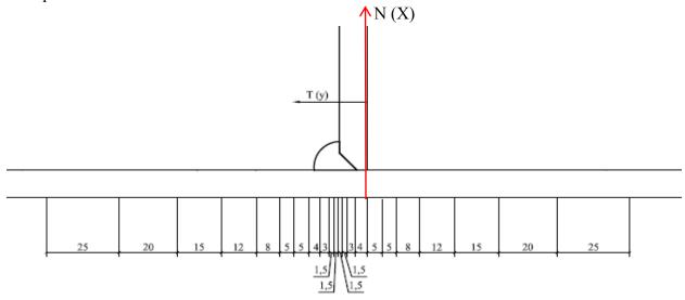
Figure 8.4: Spacing of measurements (in mm) in transverse direction on Specimen 4 (lines 1, 3, 4, 5, and 6)
