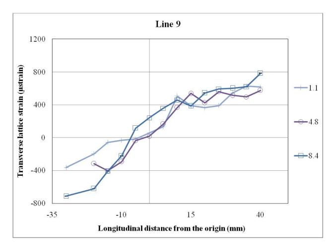
Figure 8.14: Transverse strain at various depths in the longitudinal (L) direction on line 9 (at T = 50 mm)
