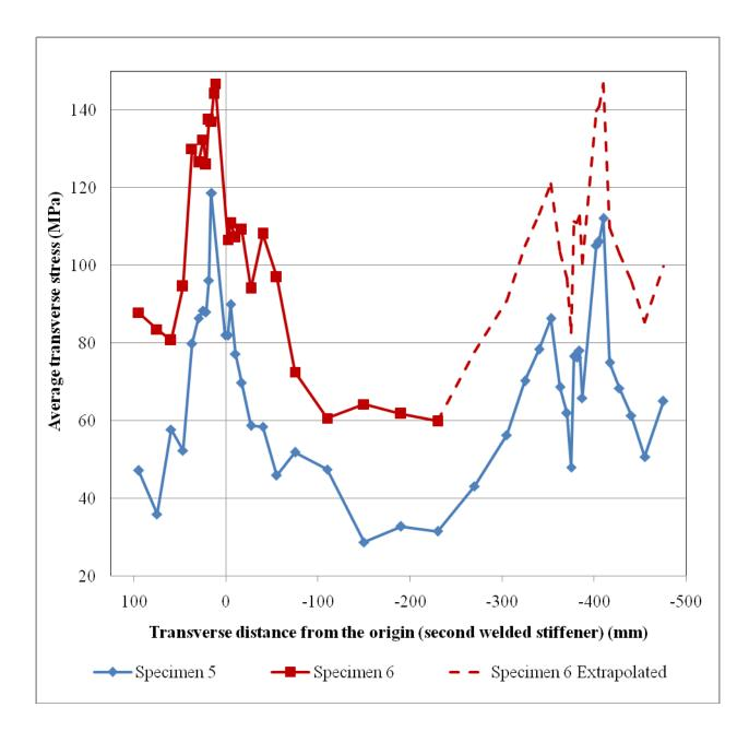
Figure 8.30: Average transverse stress distributions along the transverse lines (line 1-2-3-4 for Specimen 5 and line 1-2-3 for Specimen 6)
