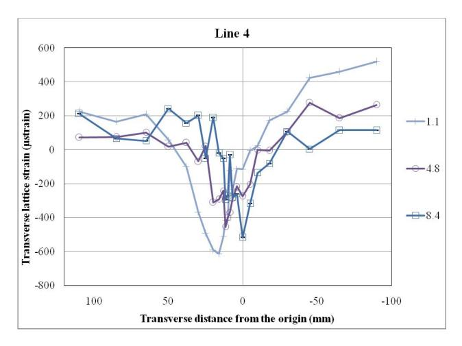
Figure 8.8: Transverse strain at various depths in the transverse (T) direction on line 4 (at L = 0 mm)
