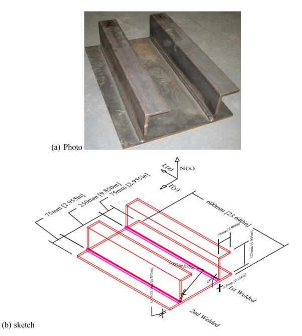
Figure 7.3: Specimen 2 (a) is a photo and (b) is the sketch
