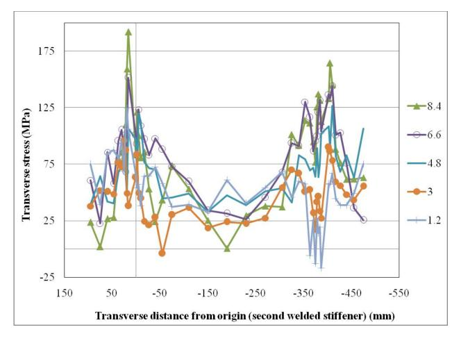
Figure 8.21: Transverse stress through the depth in the transverse (T) direction on line 1-2-3-4 (at L = 0 mm)
