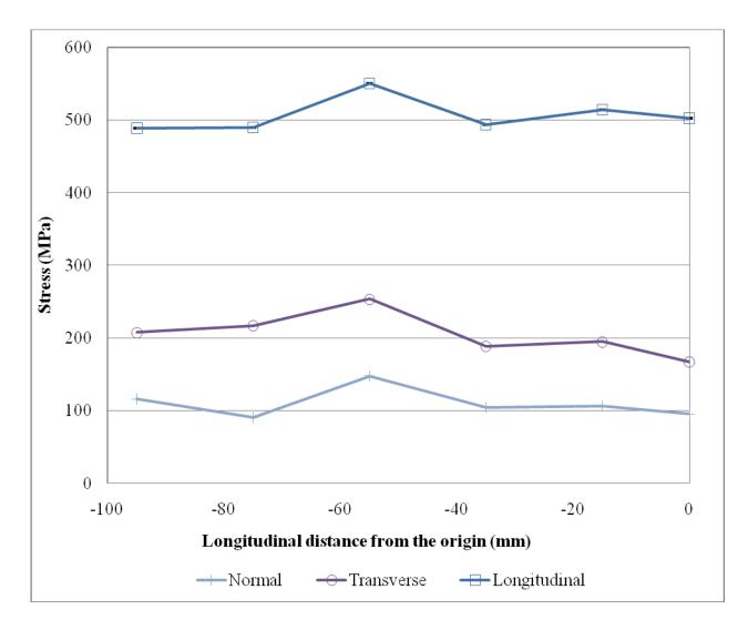
Figure 8.24: All stresses at second welded stiffener, at T = +10 mm, at N = 8.4 mm (on line 2-5)
