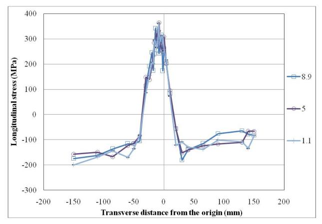
Figure 7.24: Longitudinal stress through the depth in transverse (T) direction (at L = 133 mm, line 5-2-6)
