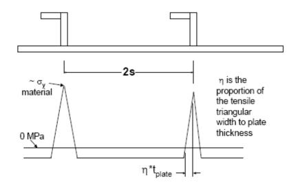
Figure 9.4: Faulkner model for residual stresses (Dexter & Pilarski, 2000)
