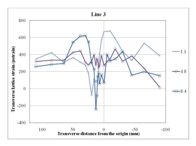
Figure 8.7: Transverse strain at various depths in the transverse (T) direction on line 3 (at L = 20 mm)
