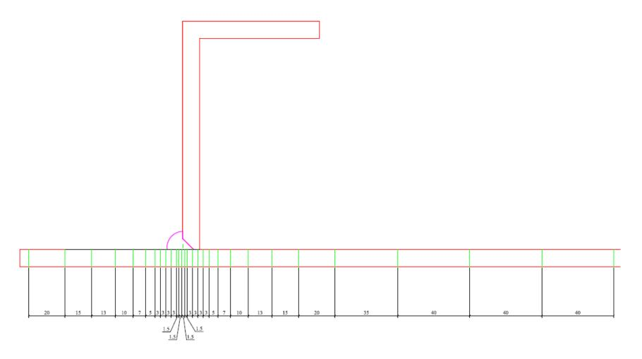
Figure 8.26: Spacing of measurements (in mm) in transverse direction for Specimen 6 (on line 1-2-3)
