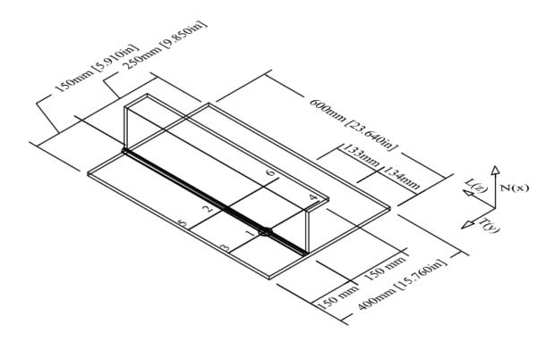
Figure 7.17: Detail for Measurement Points for Specimen 2
