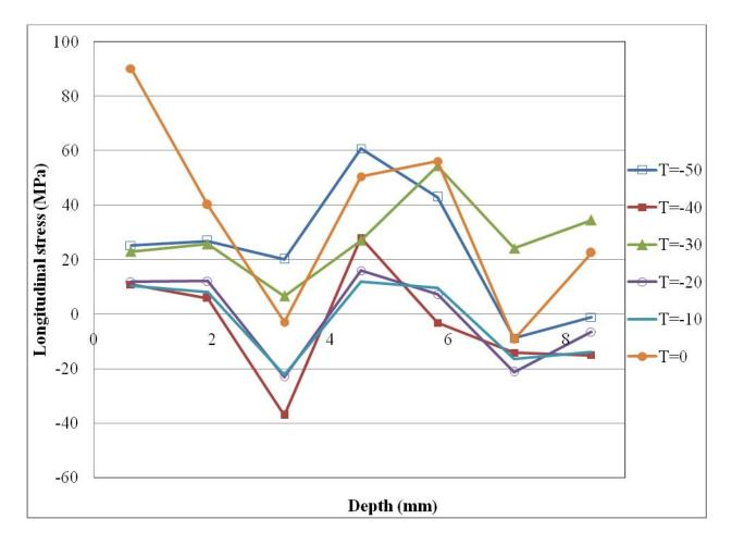
Figure 7.13: Longitudinal stress through the depth in transverse (T) direction (line 1-2)
