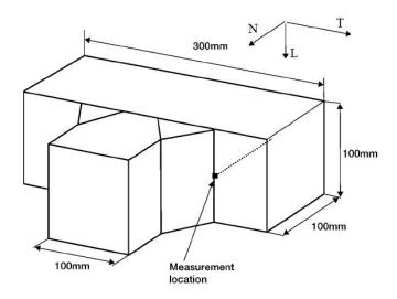
Figure 2.15: Location of deep-hole drilling measurements on the 100 mm thick plate specimen (Wimpory, et al., 2003)
