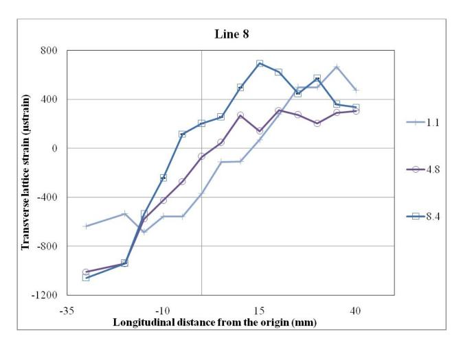
Figure 8.13: Transverse strain at various depths in the longitudinal (L) direction on line 8 (at T = 30 mm)
