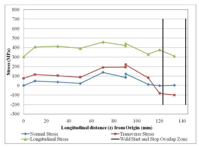
Figure 7.27: All stresses at Transverse = -10 mm, Normal = 8.9 mm (line 1-2)
