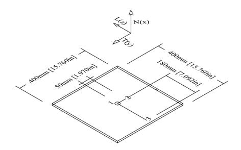
Figure 7.4: Detail for Measurement Points for Specimen 1
