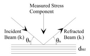
Figure 2.9: Lattice spacing with incident (k<sub>i</sub>) and refracted (k<sub>f</sub>) beam
