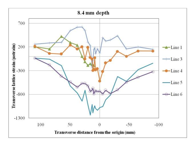
Figure 8.11: Transverse strain at a depth of 8.4 mm in the transverse (T) direction on lines 1, 3, 4, 5, and 6
