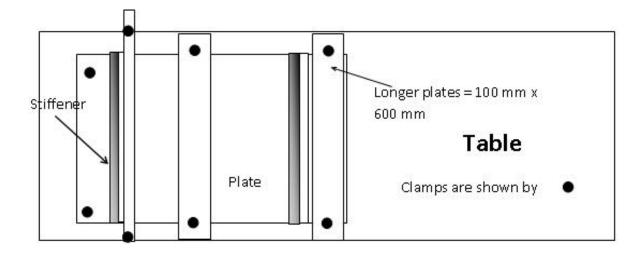
Figure 5.2: Clamp locations during welding
