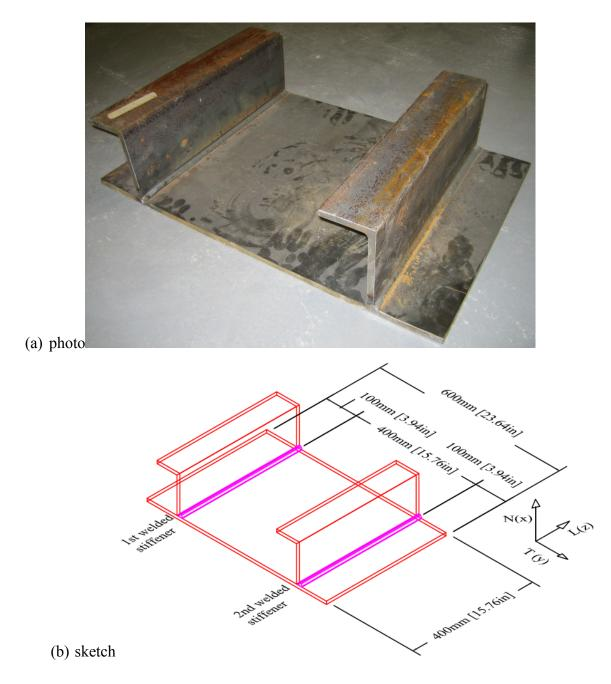
Figure 8.2: Specimens 5 and 6 (a) is a photo and (b) is the sketch
