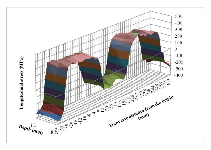
Figure 7.33: 3-D view of longitudinal stress distribution in transverse (T) direction (line 2-1-3)
