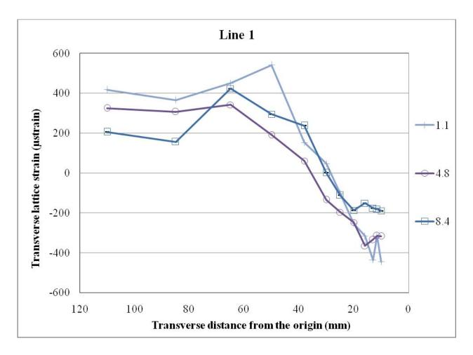
Figure 8.5: Transverse strain at various depths in the transverse (T) direction on line 1 (at L = 200 mm)
