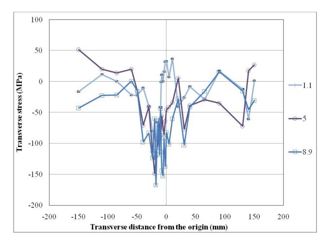
Figure 7.22: Transverse stresses through the depth in transverse (T) direction (at L = 133 mm, line 5-2-6)
