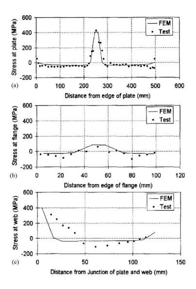
Figure 2.2: (a) Distance from edge of plate (mm) vs. Stress at plate (MPa); (b) Distance from edge of flange (mm) vs. Stress at flange (MPa); (c) Distance from junction of plate and web (mm) vs. Stress at web (MPa). (Hu & Jiang, 1998)
