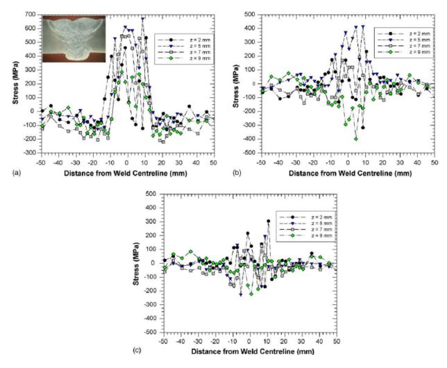
Figure 2.12: Specimen - 12 mm thick, overmatched weld metal at low heat input 1kJ/mm (a) Longitudinal (x) stress profile at four depths (b) Transverse (y) stress profile at four depths (c) Through-thickness (z) stress profile at four depths (James, et al., 2006)
