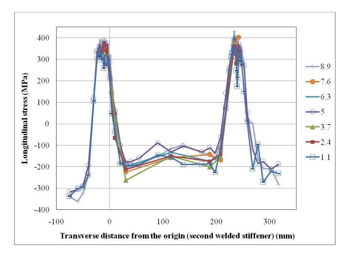
Figure 7.32: Longitudinal stresses through the depth in transverse (T) direction (line 2-1-3)
