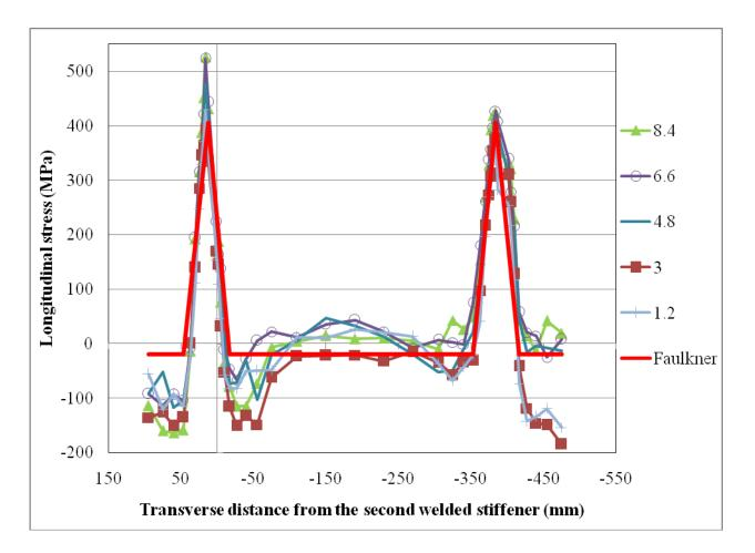
Figure 9.6: Specimen 5, two stiffeners spaced at 400 mm, high heat input
