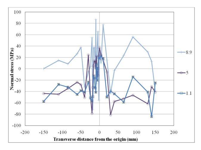
Figure 7.20: Normal stresses through the depth in transverse (T) direction (at L = 133 mm, line 5-2-6)
