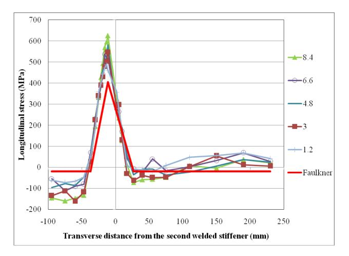
Figure 9.7: Specimen 6, two stiffeners spaced at 400 mm, moderate heat input
