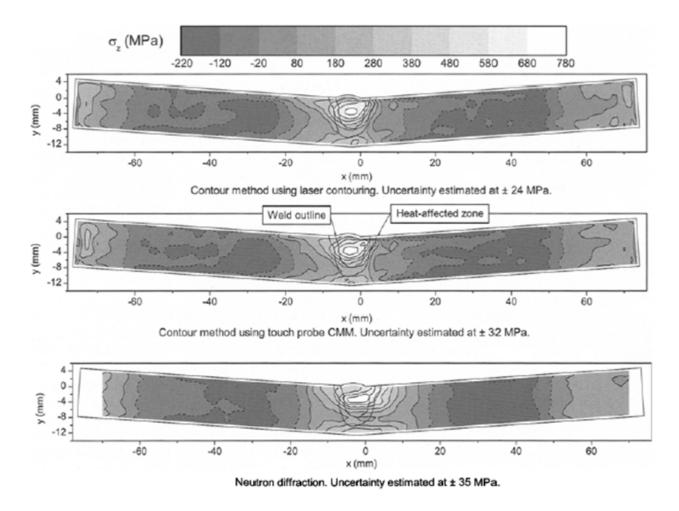
Figure 2.3: The stress maps measured with the contour method and neutron diffraction (Prime, et al., 2004)
