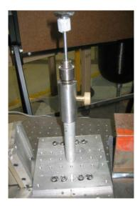
Figure 6.5: Nickel-reference sample in cadmium container
