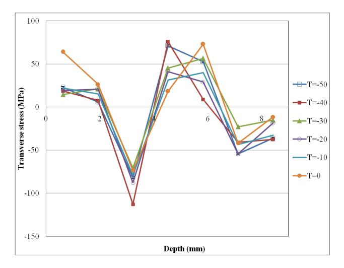
Figure 7.9: Transverse stress through the depth in transverse (T) direction (line 1-2)
