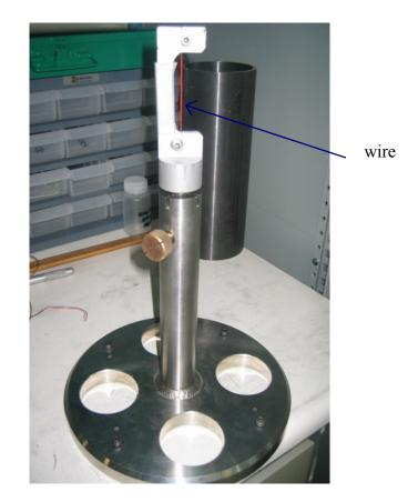
Figure 6.3: Wire mount used to sight centre of rotation with telescopes
