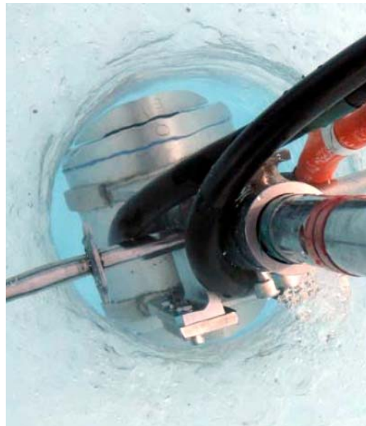
Figure 3.8: Borehole Jack for In-Situ Compression Test in Ice (Source: Photo by Lanthier from Timco and Weeks, 2010)
