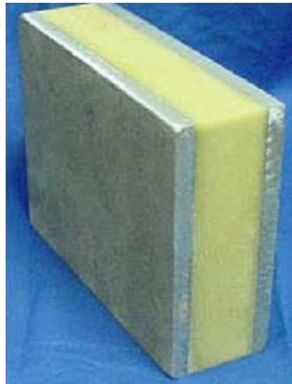
Figure 3.27: Sandwich Plate System (SPS)
