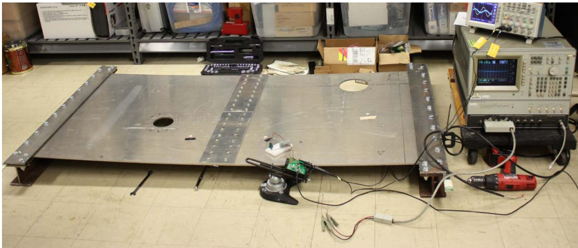
Figure 21. The base plate is placed in end clamps to supply fixed-fixed boundary conditions. The HP 4194A impedance analyzer is shown in the right of the picture.
