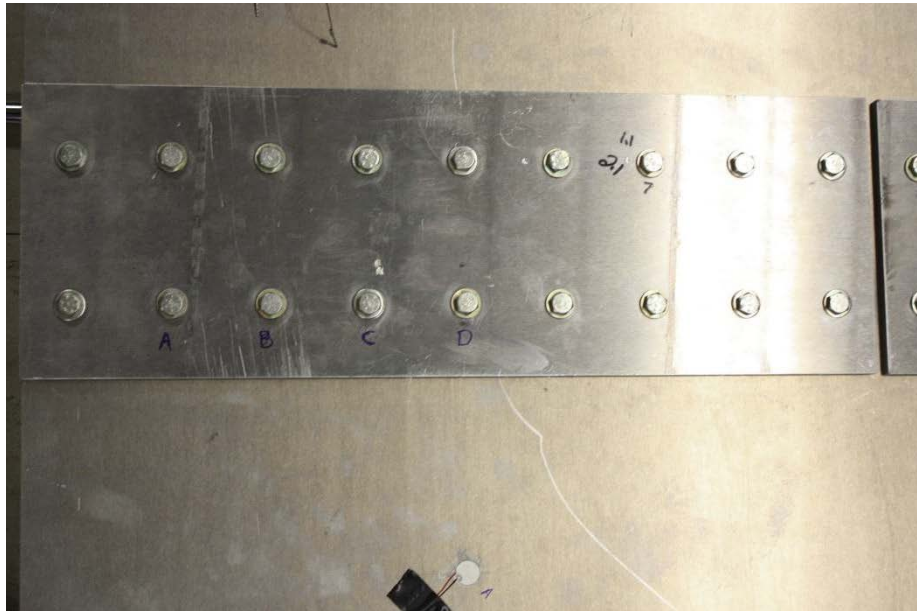
Figure 22. The left doubler, piezo disc, and loosened bolt labels are displayed.
