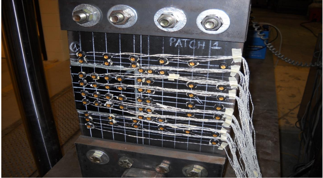
Figure 6-12. Front view of the plate with a flexible patch and location of markers
