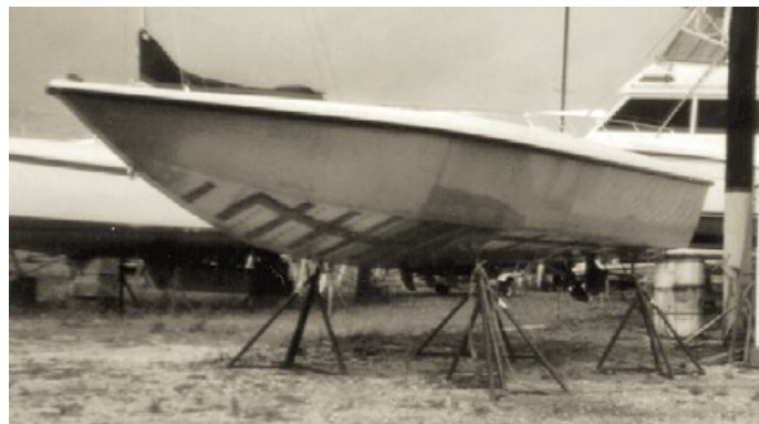
Figure 16 Recreational Ski Boat. Translucent hull makes location of manometer taps visible in this view. Figure reproduced from Royce (2001).
