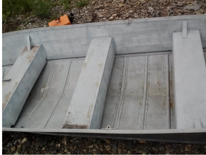
Figure 29 Structure of aluminum fishing boat. Transverse stiffeners are visible on the hull.
