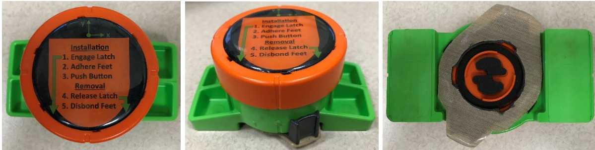
Figure 4. Top, side, and bottom views of the structural sonar installation tool
