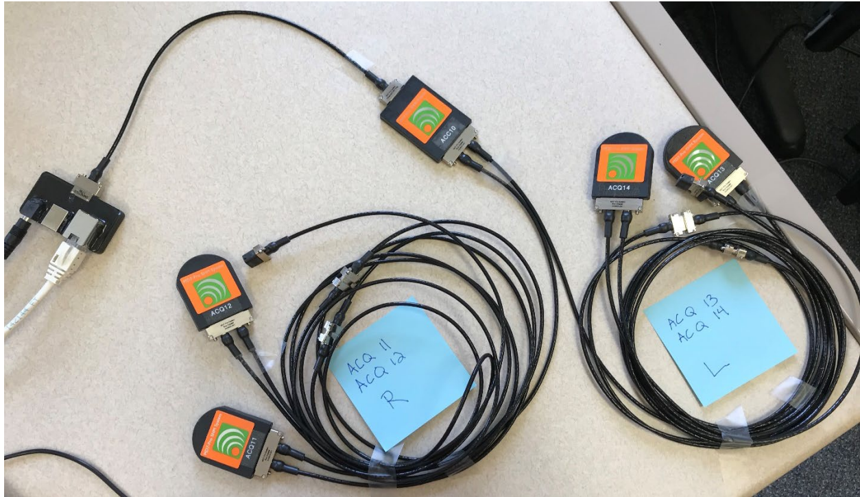
Figure 2. The MD7-Pro bus assembly prior to structural sonar attachment
