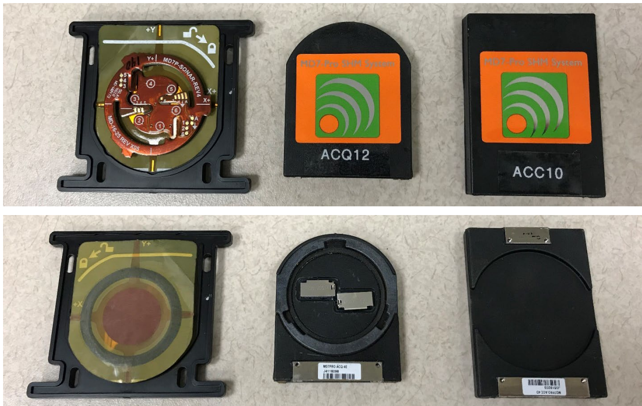
Figure 1. The MD7-Pro structural sonar (left), acquisition node (center), and accumulator node (right)
