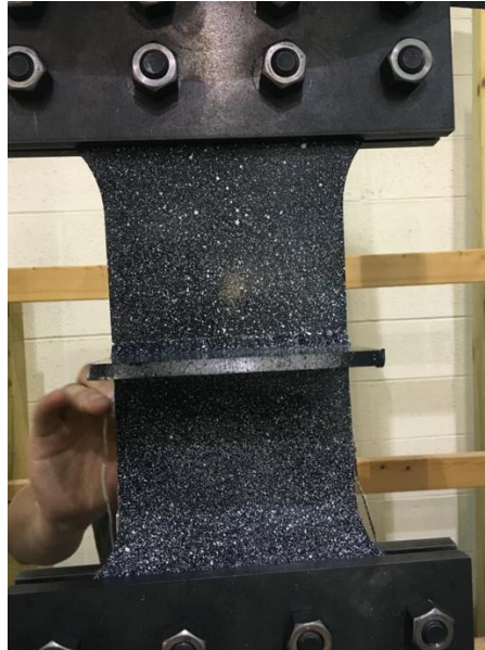
Figure 40: Specimen C1 Before Testing
