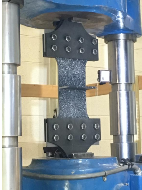
Figure 29: Specimen A1 Before Testing
