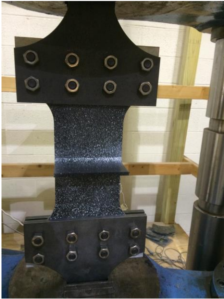
Figure 31: Specimen A2 Before Testing
