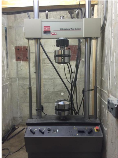
Figure 15: MTS 810 Machine Used for Material Coupon Testing
