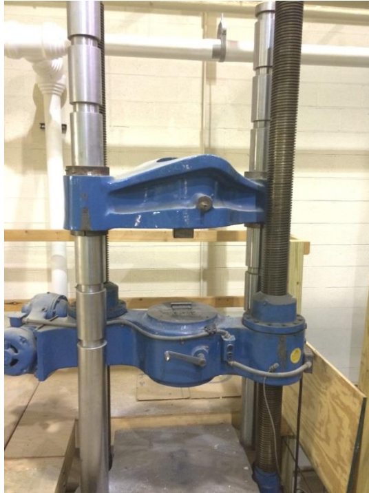
Figure 17: Load Frame for Large Specimen Tests
