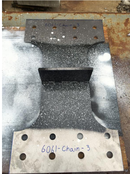
Figure 54: Specimen E3 Before Testing
