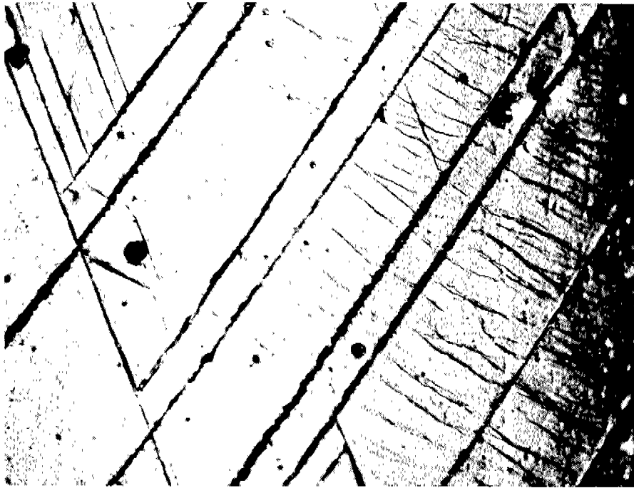
Fig. 56. Slip lines (wavy) and twins (heavy straight lines), in specimen A-11 tested at -196^{\circ}\text{C} (X150)
