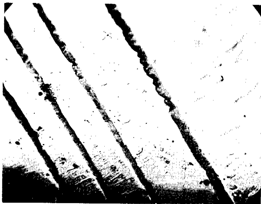
Fig. 68. Twin faces (dark bands) at high resolution showing the notching effect (X1000).
