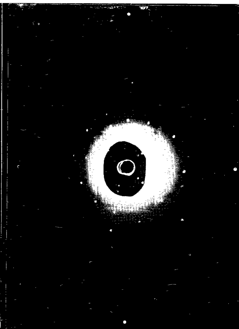
Fig. 63. Laue photograph of specimen A-1 taken after 5 percent elongation. Note splitting of spots and rotation of crystal axis.
