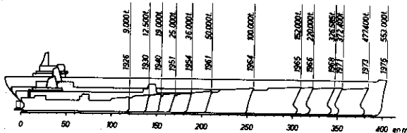
Fig. 1 - Increase of the DWT of tankers in the last years
