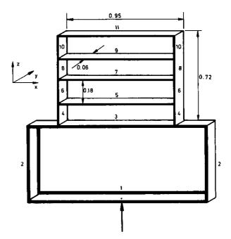
Scale model for measurements Fig. 7. of the attenuation of structure-borne sound. The thickness of the plates 1 - 3 is 1 mm and of the plates 4 - 11 0.6 mm. Other dimensions in m.
