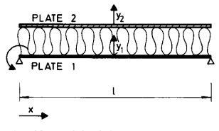
Fig. 15. Model of floating floor.
