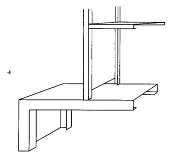
Fig. 8. Scale model 6. The superstructure connected to the main deck via the frames.
