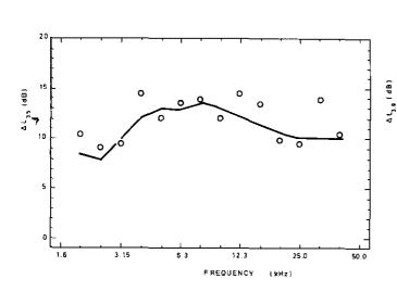
Fig. 12. Velocity level differences between the plates 3 and 5 for model 2.
