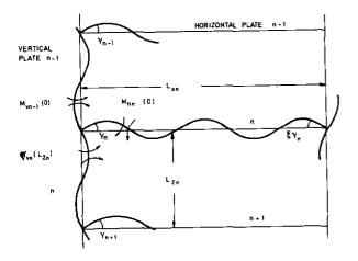
Fig. 4. Resulting bending moments and angular displacements at a Tjunction.
