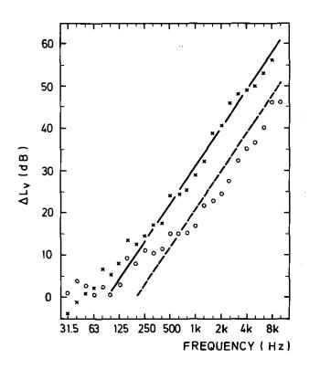
Fig. 17. Velocity level differences between the bottom and top plates. For type C floor solid line is calculated result and x line is the measured result. The dashed line an O line are the corresponding results for the D construction.
