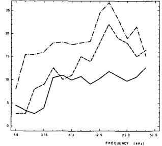
Fig. 13. Measured velocity level differences between the plate elements 3 and 5.
