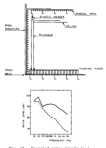
Fig. 18. Measured noise levels in a cabin above the propeller. The solid line is the level when bulkheads and ceiling are mounted firmly to the steel decks. The dashed line is the result for the floating accommodation system shown above.
