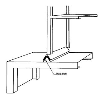
Fig. 9. Scale model 7. The superstructure is elastically mounted on the main deck.
