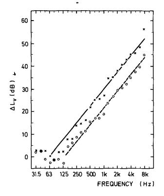
Fig. 16. Velocity level differences between the bottom and top plates. For type A floor solid line is calculated result and x line is the measured result. The dashed line and O line are the corresponding results for the B construction.
