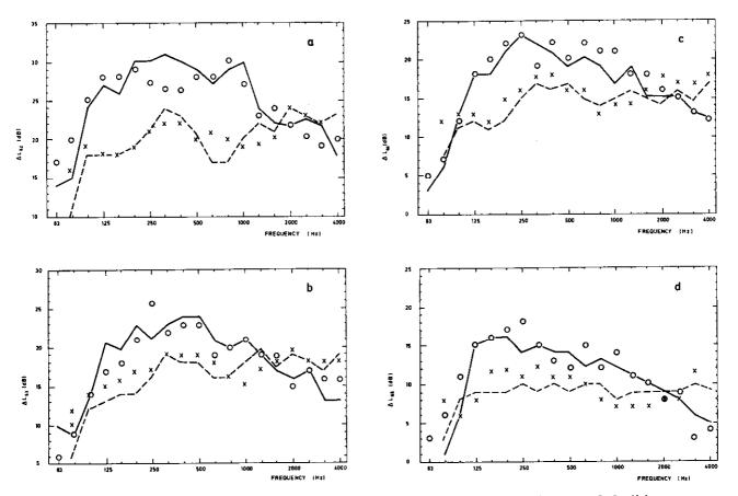
Fig. 6. Velocity level differences between the decks 6 and 2 (a), 6 and 3 (b), 6 and 4 (c), 6 and 5 (d) Compare Fig. 3.
