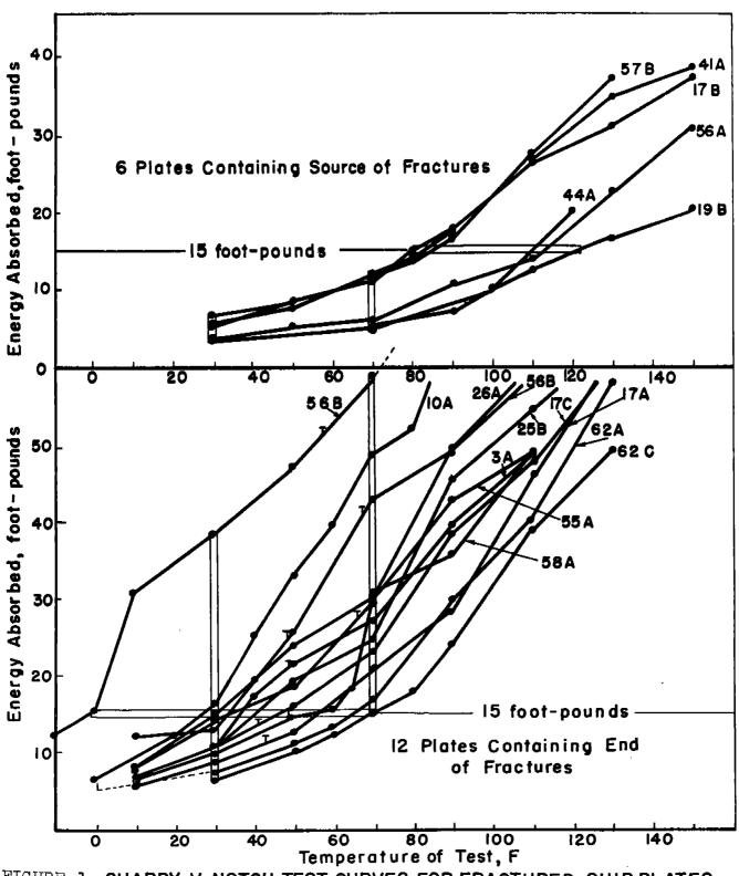
FIGURE 1. CHARPY V-NOTCH TEST CURVES FOR FRACTURED SHIP PLATES, 0.44-0.69 INCH THICKNESS
