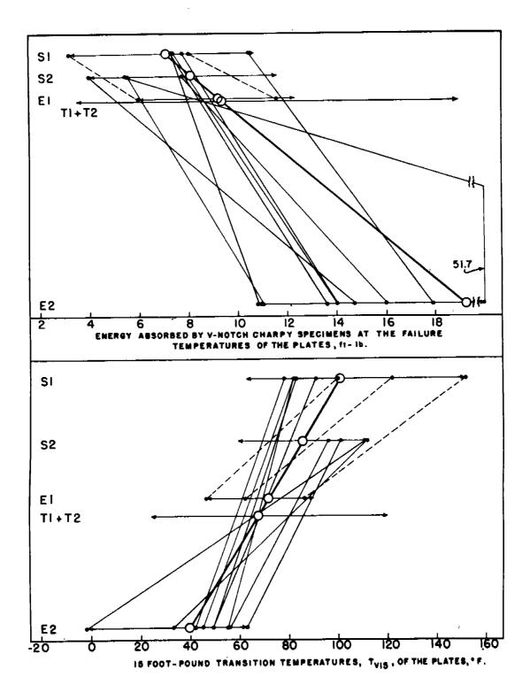
Fig. 3. Notch sensitivity of source and end plates from same ship, compared to ranges and average values for the different fracture categories. The fracture categories are spaced vertically so that the average values (large circles) fall on the heavy line. Other diagonal lines indicate relative values for pairs of source (SL or S2) and end (EL or E2) plates from the same ship. Morizontpl arrows show the range of values for all plates in each category.
