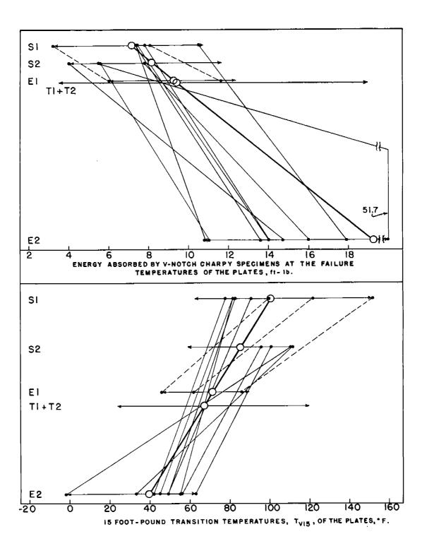
Fig. III.3. Notch sensitivity of source and end plates from same ship, compared to ranges and average values for the different fracture categories. The fracture categories are spaced vertically so that the average values (large circles) fall on the heavy line. Other diagonal lines indicate relative values for pairs of source (Stor S2) and end (Etor E2) plates from the same ship. Horizontpl arrows show the range of values for all plates in each category.
