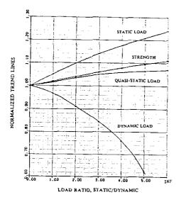
Figure 7 Trends of Partial Safety Factors with the Ratio of Static to Dynamic Loads in TLP Flat Plate Structures.
