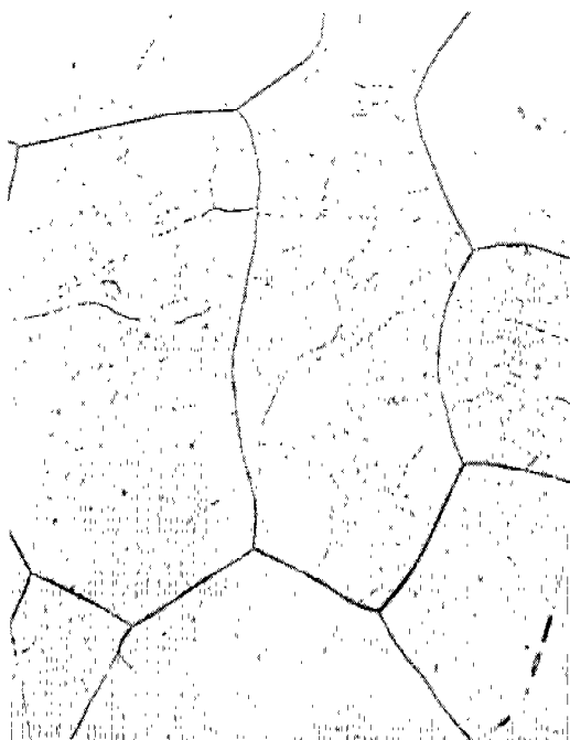
Figure 17. Alloy 98V, .0059% C. Furnace cooled from 1000 C. Different view of specimen of Fig. 16, heavily etched with Picral to bring out veining of ferrite. 200 X
